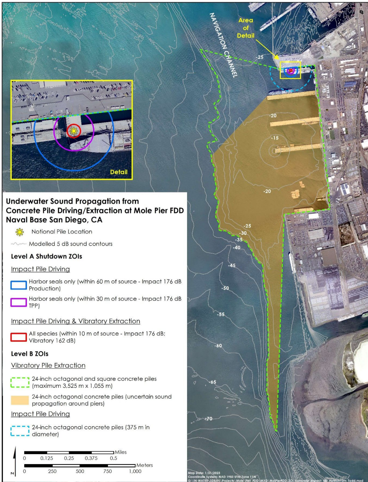
Figure 3--3. Underwater Sound from Impact Pile Driving Using a Site-Specific Model.
