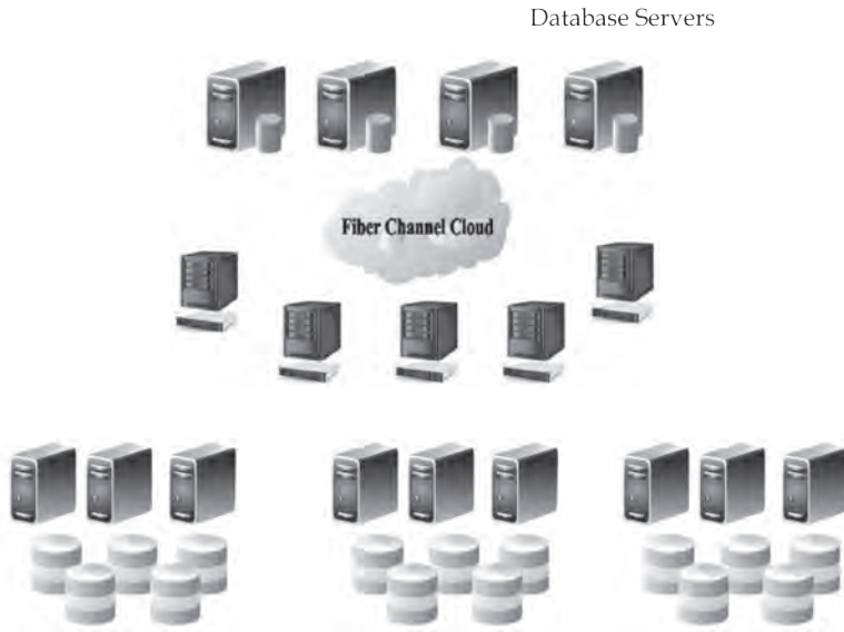
Figure 8.5. Elements of Storage Area Networks.
