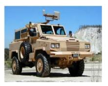
**Specifications.** Protection from Mine/UXO/IED Blast, Ballistic Protection, High Protected Mobility, 4x4 Configurations, Turret Weapon Mountable.
