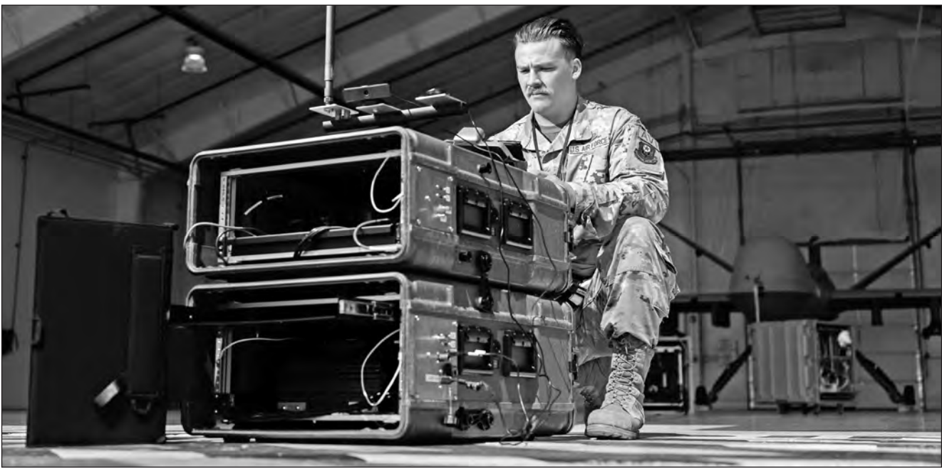
Staff Sgt. Chase Ward, 727th Special Operations Aircraft Maintenance Squadron avionics craftsman, operates the third generation of the digital aircraft link emulator in front of an MQ-9 Reaper remotely piloted aircraft, and two older generations of DALE on Cannon Air Force Base, New Mexico, Aug. 25. Master Sgt. Bridget Carroll created DALE seven years ago to reduce the size of RPA maintenance packages loaded onto cargo aircraft when deploying. (U.S. Air Force photo by Staff Sgt. Candin Muniz)
