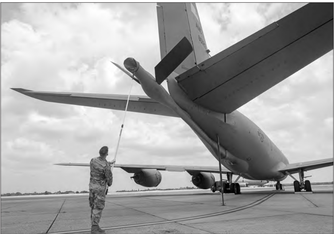
Airman 1st Class Jacob Helzer, 100th Maintenance Squadron hydraulics maintenance journeyman, uses the Boom Cover Tool on a KC-135 Stratotanker aircraft at RAF Mildenhall, United Kingdom, July 22. The Boom Cover Tool, created by Helzer, is expected to save 40,000 man-hours and $1 million annually. (U.S. Air Force photo by Airman 1st Class Alvaro Villagomez)
