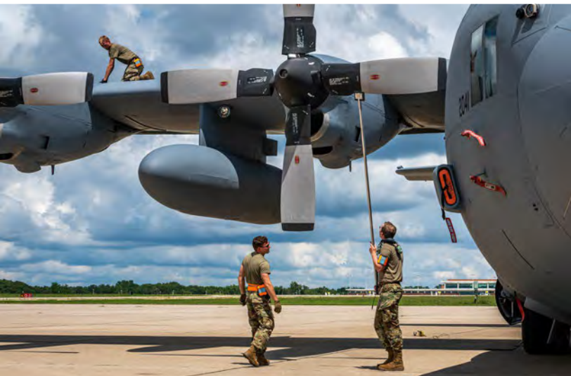
U.S. Air Force Airman 1st Class Chance Whisenand, a crew chief assigned to the 182nd Aircraft Maintenance Squadron, Illinois Air National Guard, performs a post-flight wing walk on a C-130H Hercules at the 182nd Airlift Wing in Peoria, Illinois, Aug. 14, 2022. The 182nd maintains and operates C-130H Hercules aircraft capable of airlifting and airdropping personnel and equipment.
