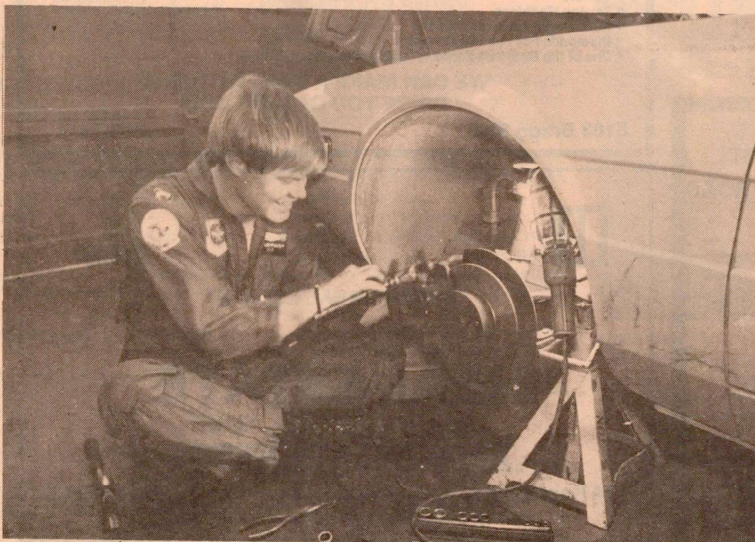
1st Lt. Brian Lightwardt repairs disc brakes
