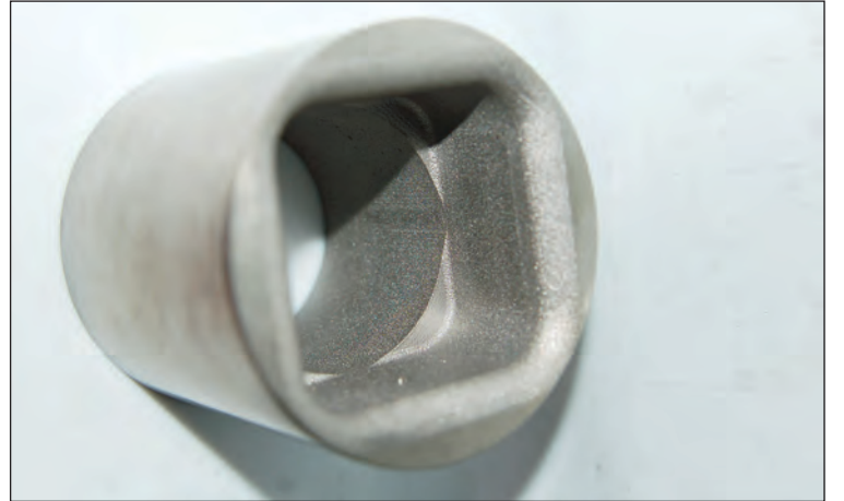
Pictured is a petal orifice liner created at Arnold Engineering Development Complex Hypervelocity Wind Tunnel 9 in White Oak, Maryland, using additive manufacturing, otherwise known as 3D printing. The refractive metal part has an outside diameter of around 3 inches, an inside diameter of around 2 inches and is nominally 3 inches in length. (U.S. Air Force photo)
