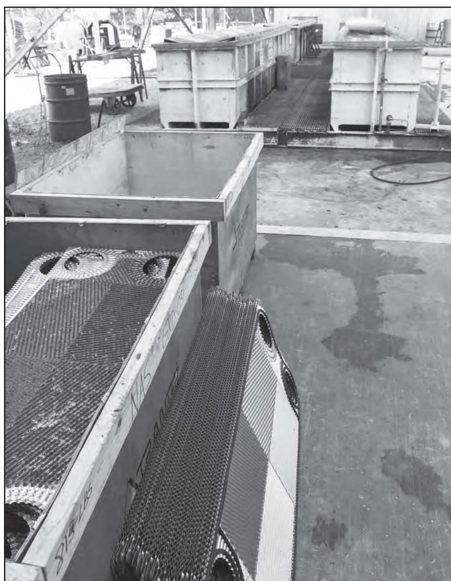
In the foreground sit stacks of parts from a test facility at Arnold Air Force Base June 29 showing the before and after states of chemical cleaning operations. The parts in the box are before cleaning. The parts leaning against the box have been cleaned. One of the steps in the process uses newly-acquired citrus-based cleaners, which were purchased to replace a significantly more hazardous chemical, hydrofluoric acid. (U.S. Air Force photo by Jill Pickett)
