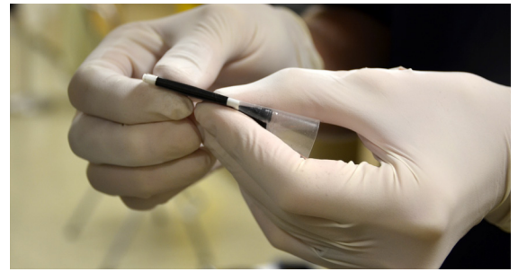
Wright-Patterson AFB, Ohio. Flexible lithium-ion batteries developed by researchers at the Air Force Research Laboratory have the potential to power countless flexible electronic devices, including human performance sensors and flexible displays, and are able to maintain a steady voltage discharge following extreme mechanical stress testing. U.S. Air Force Photo by Marisa Alia-Novobilski. October 4, 2016.
