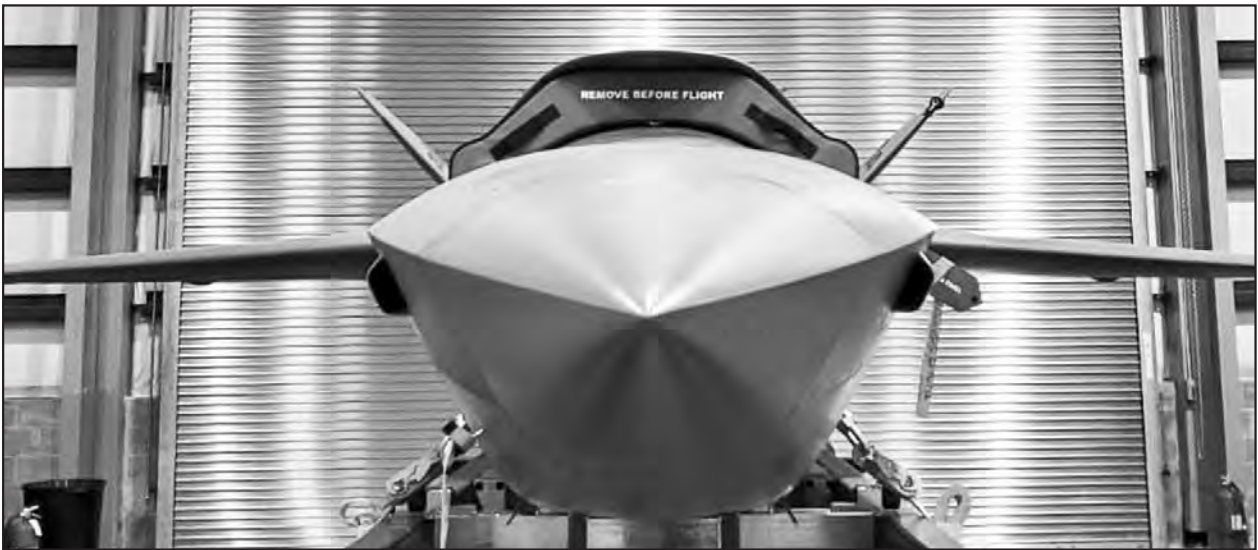
The 40th Flight Test Squadron took possession of the first of two government-owned Kratos XQ 58A Valkyrie aircraft. The Valkyrie is a low-cost, high-performance uncrewed air vehicle. It is rocket-launched off a rail system and is controlled from a ground station or airborne fighter. An onboard computer system is capable determining the best flight path and throttle settings to comply with commands. (Courtesy photo)
