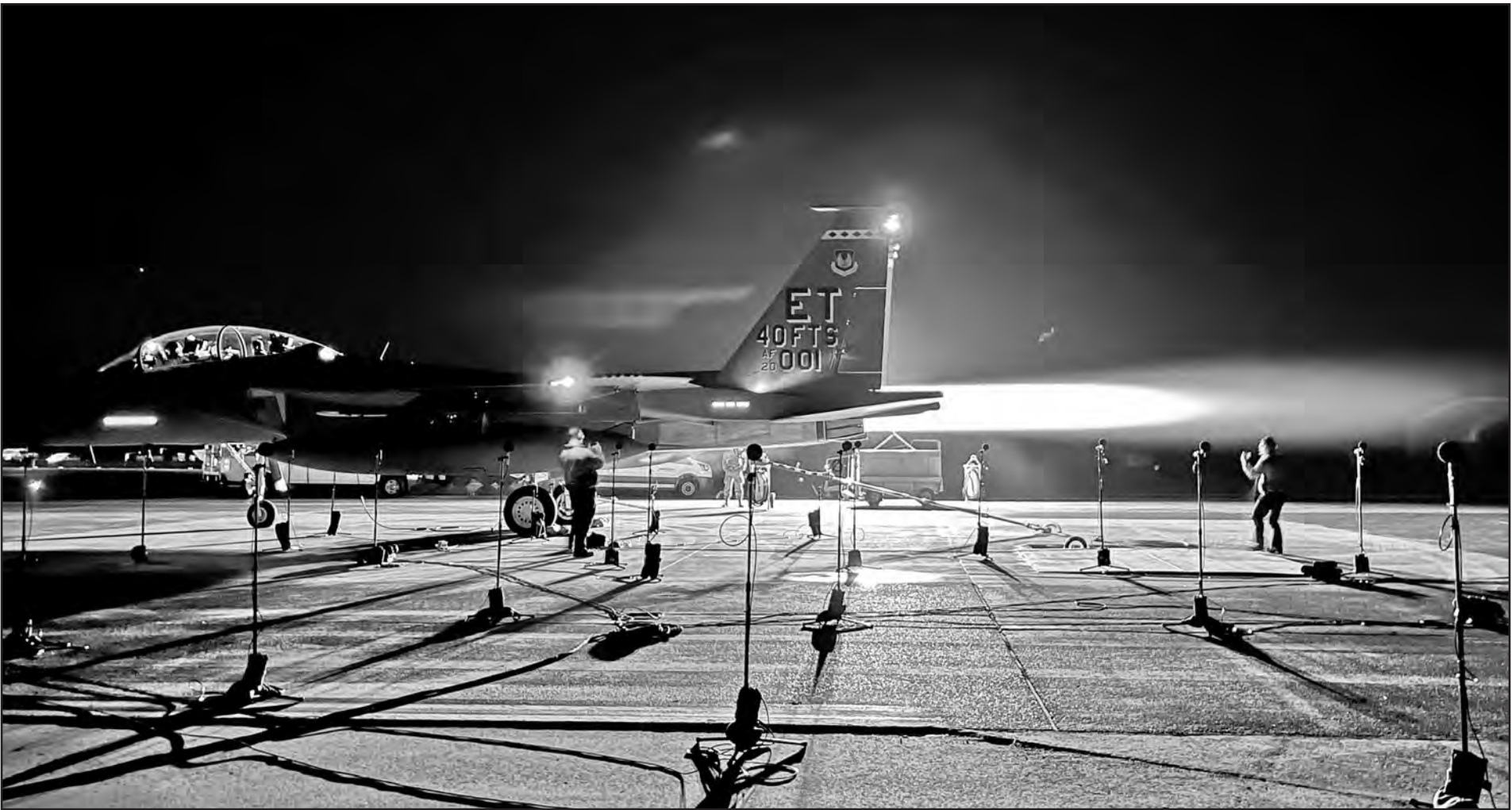
Microphones record the sounds of the F-15EX Eagle II’s engines during a ground test Oct. 26 at Eglin Air Force Base, Florida. The aircraft underwent various ground and flight acoustic testing to create a baseline noise level for use by the Department of Defense. This was the first time this type of in-depth digital acoustic sound testing was done on any F-15 model. (U.S. Air Force photo)
