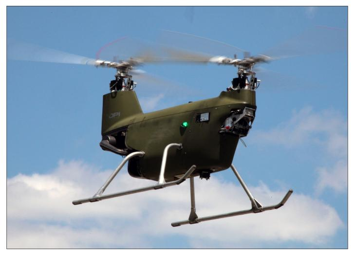
The DP-12 Rhino, above, is designed for Humvee-based transportable vertical take-off and landing (VTOL). The DP-6 Whisper, next page, is the first electric tandem UAV.
