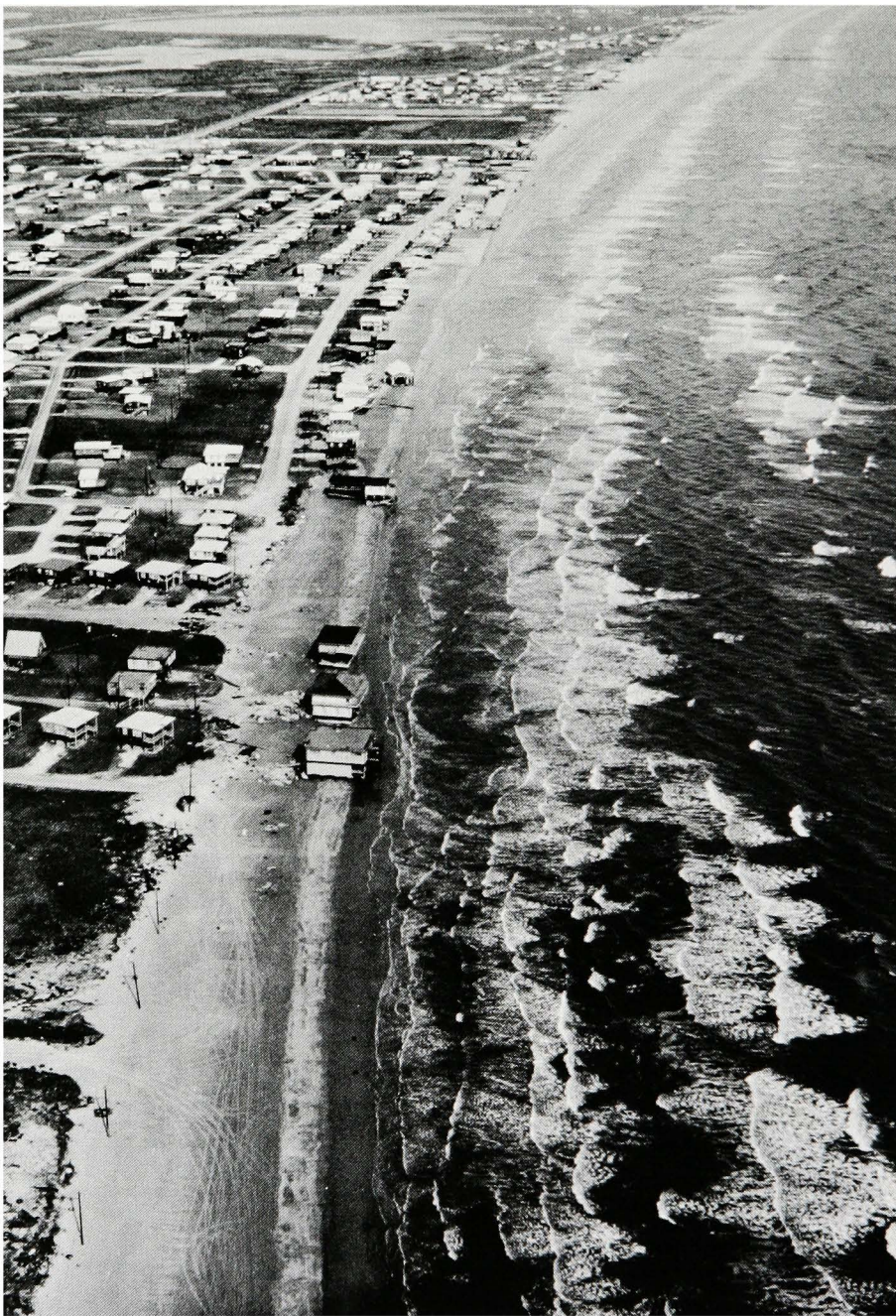
Dramatic beach erosion at Surfside is now being studied by the Corps. Note road washed out behind houses where beach has already disappeared.
