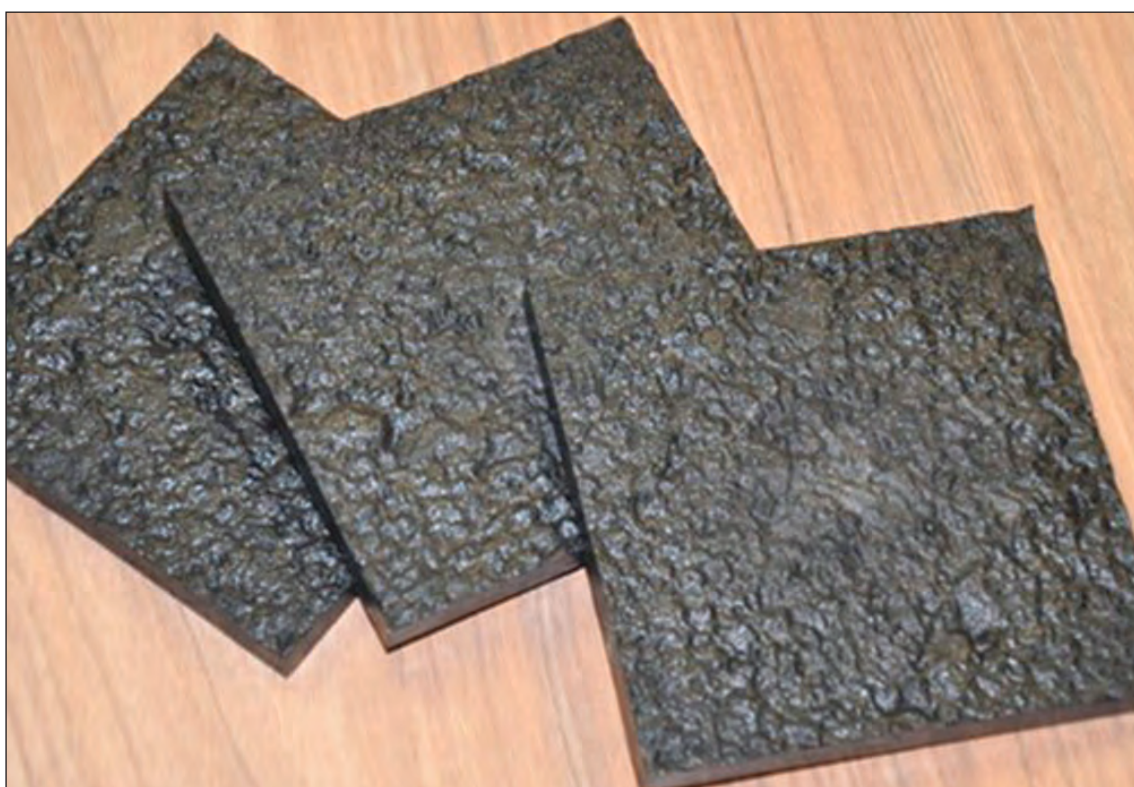
Additively manufactured tiles produced by Open Additive, LLC, such as those shown, for use in the 168-inch internal drum dynamometer at the Landing Gear Test Facility at Wright-Patterson Air Force Base, Ohio, are being developed and produced through a Small Business Innovative Research contract. A complete usable tile for use in the dynamometer is expected within the year. (Courtesy photo)
