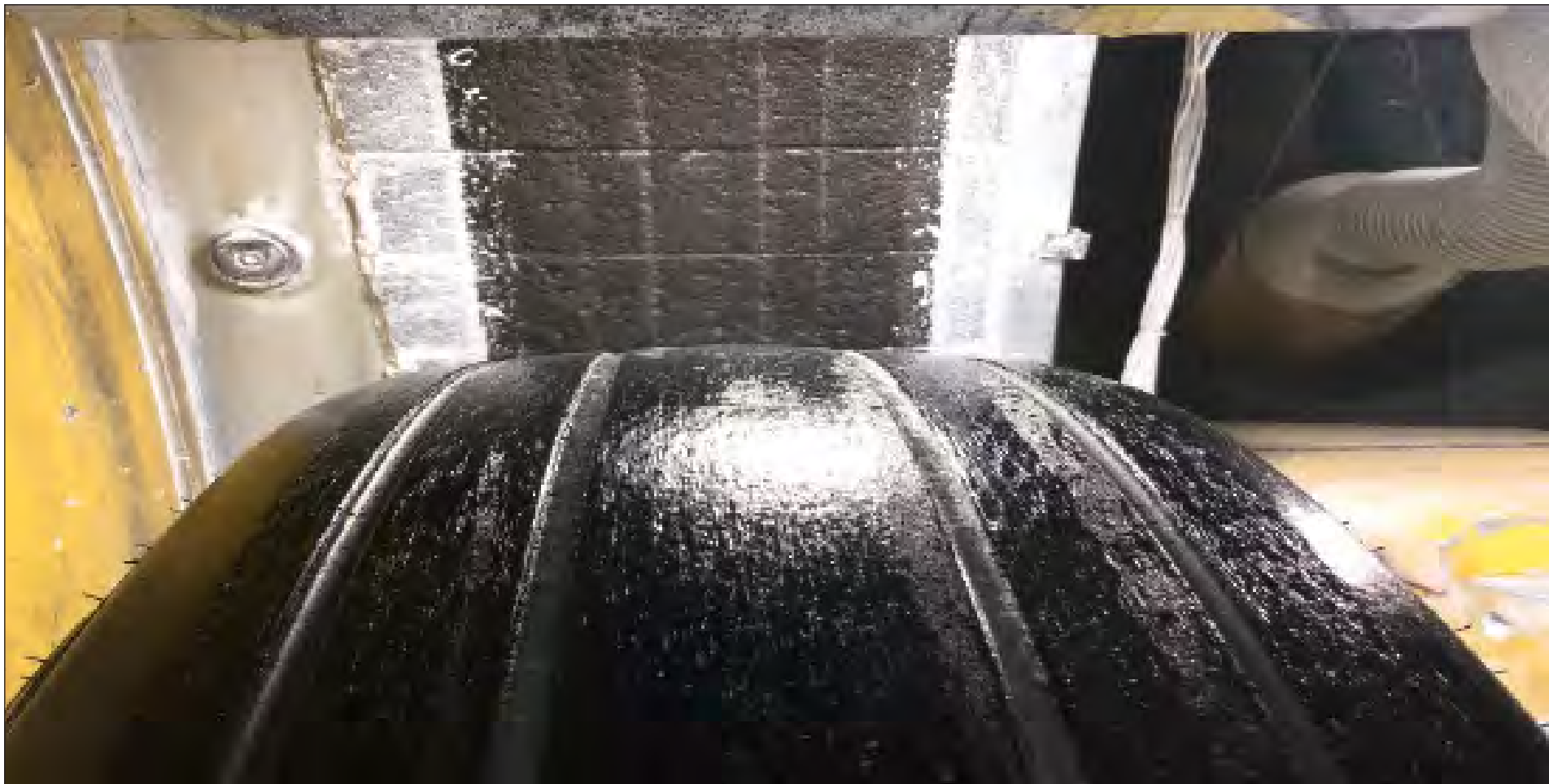
A tire undergoes Missionized Tire Wear Testing in the 168-inch internal drum dynamometer at the Landing Gear Test Facility at Wright-Patterson Air Force Base, Ohio, with concrete tiles installed to simulate a specific runway surface. The concrete tiles are created by taking molds of a runway then casting the tiles. The dynamometer operates at speeds up to 350 mph, with loads of up to 150,000 pounds, plus or minus 20 degrees of yaw, plus or minus 10 degrees of camber and can provide variable levels of brake torque. (U.S. Air Force photo)
