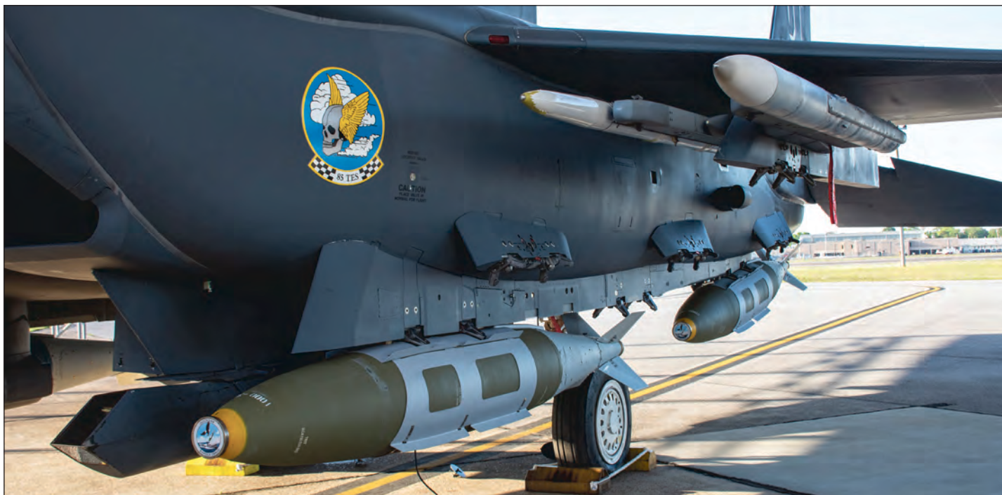
The Air Force Research Laboratory partnered with the 780th Test Squadron of the 96th Test Wing and the 85th Test and Evaluation Squadron of the 53rd Wing to equip the F-15E Strike Eagle at Eglin Air Force Base, Fla., with modified 2,000-pound GBU-31 Joint Direct Attack Munitions as part of the second test in the QUICKSINK Joint Capability Technology Demonstration. Eglin’s Integrated Test Team demonstrated QUICKSINK, a new low-cost, air-delivered capability for defeating maritime threats April 28 successfully destroying a full-scale surface vessel in the Gulf of Mexico. (U.S. Air Force photo by 1st Lt Lindsey Heflin)
