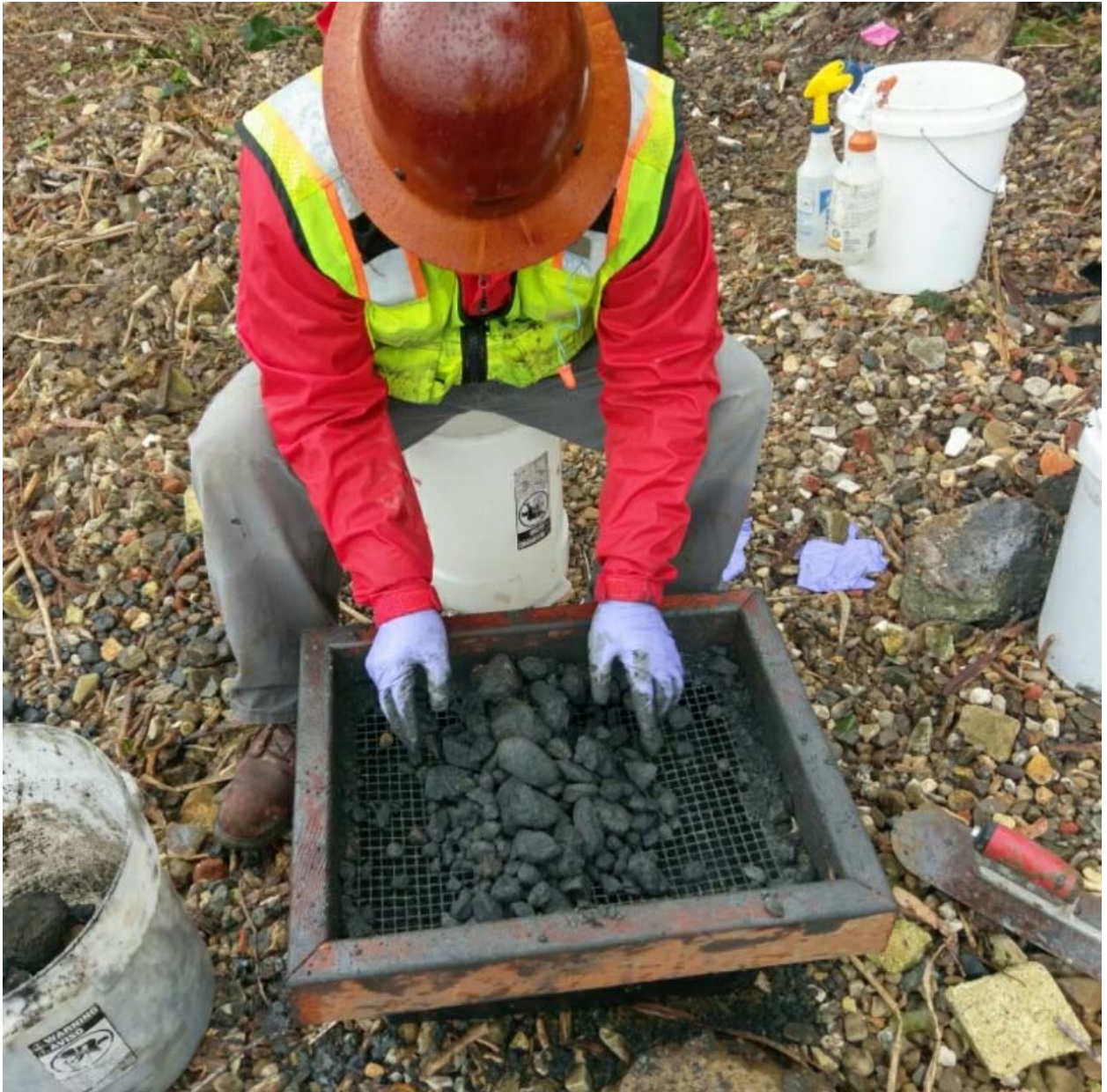
Photograph 3. Sieving the bioassay sediment.
