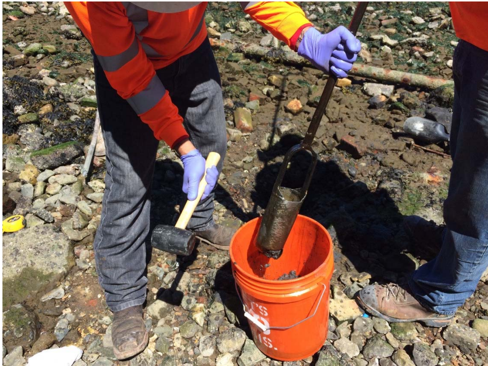
Photograph 2. Extracting subsurface sediment from hand auger barrel into bucket.
