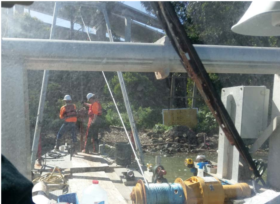
Photograph 2. Retrieving the sediment sample at location YF322 using Vibracore technology from the sampling barge.
