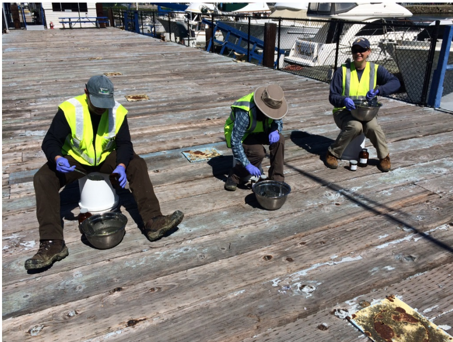
Photograph 2. Homogenizing sediment from all three depth intervals.
