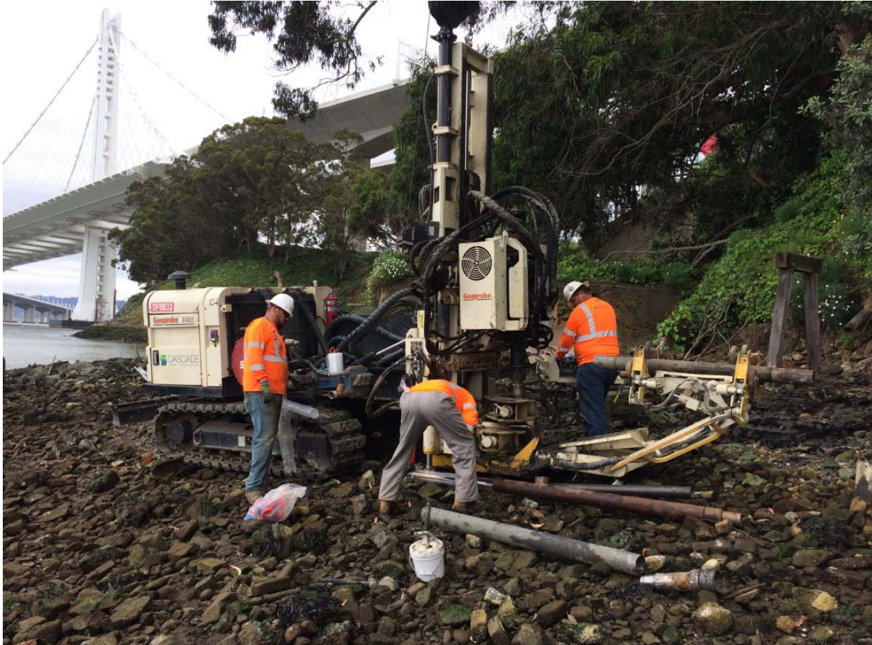
Photograph 5. Preparing to collect sediment core using hard liner at YF308.
