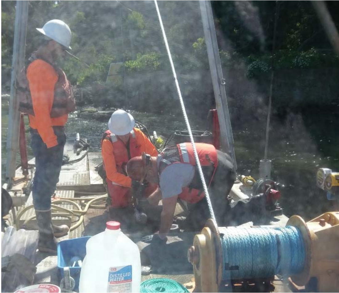
Photograph 3. Labelling the retrieved sediment core at location YF322.
