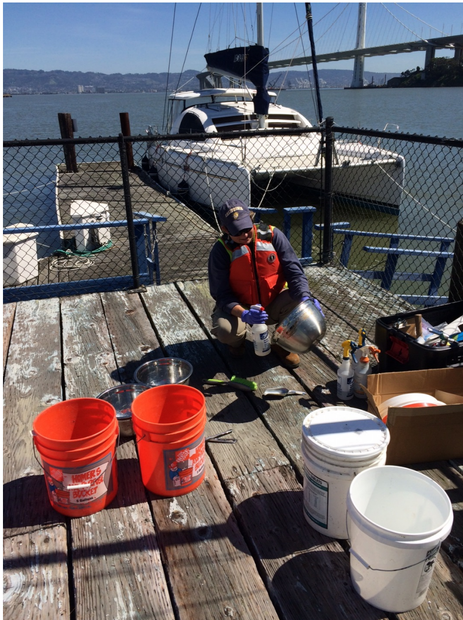
Photograph 3. Decontaminating the homogenization bowls.
