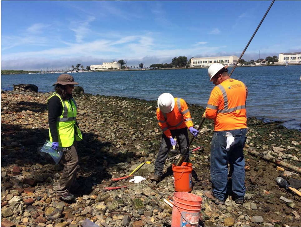
Photograph 1. Collecting subsurface sediment samples at location YF315.
