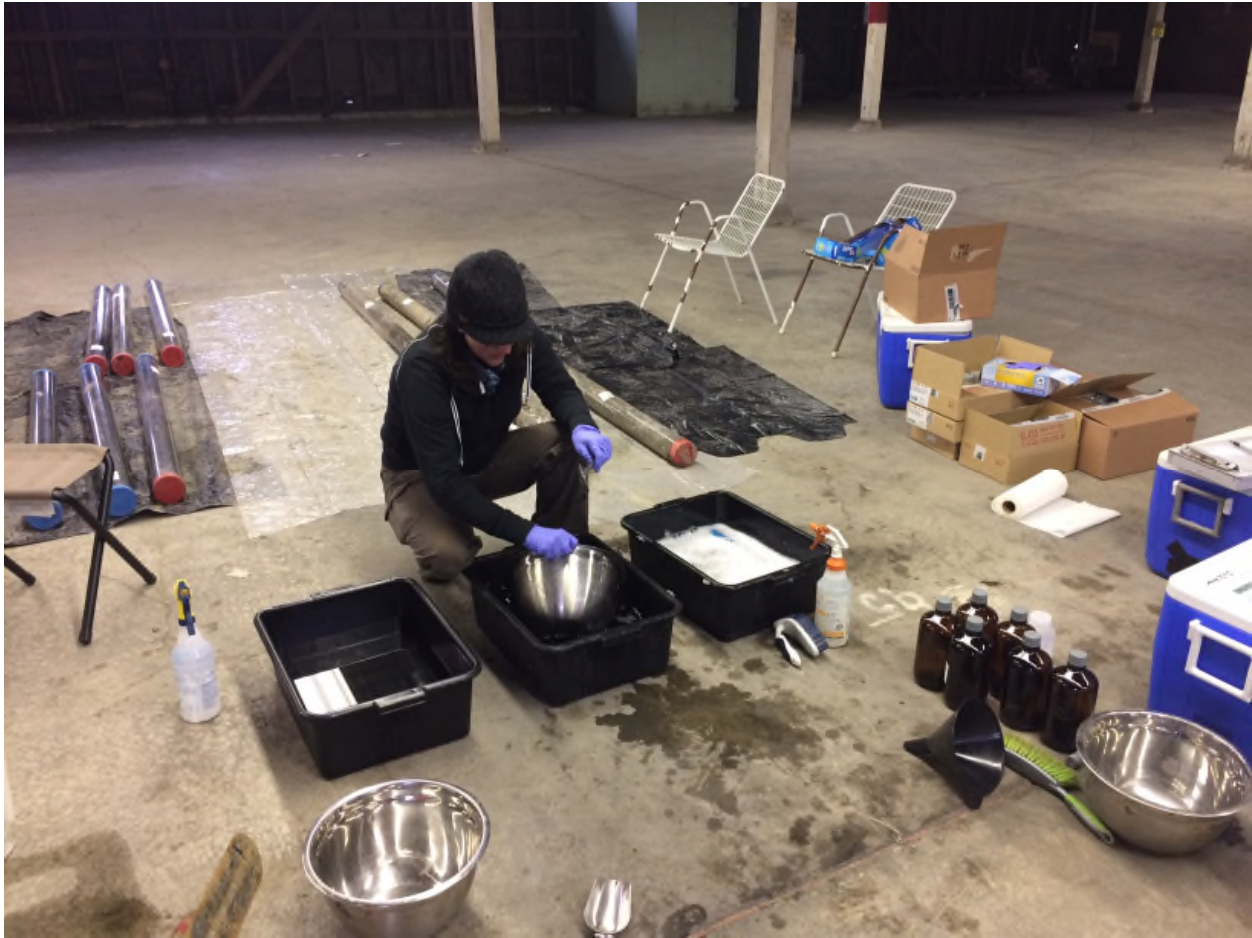
Photograph 1. Decontamination of sampling equipment in Building 96.
