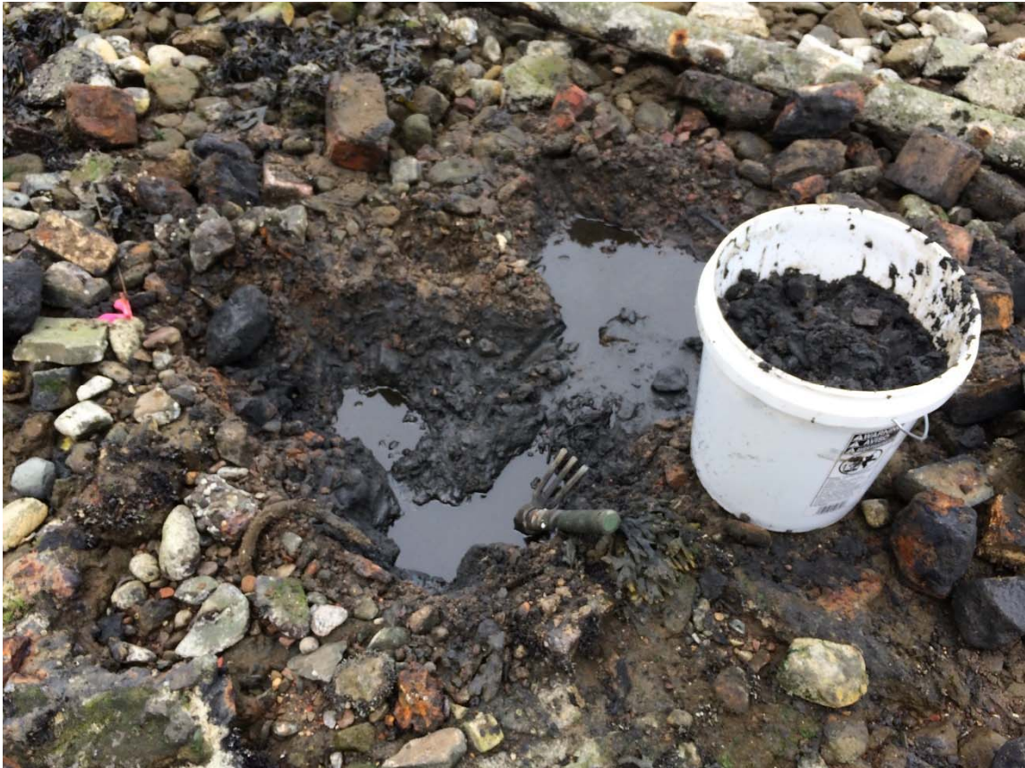
Photograph 2. Collecting the sediment sample for bioassays (0 to 1 feet below surface) at location YF315.
