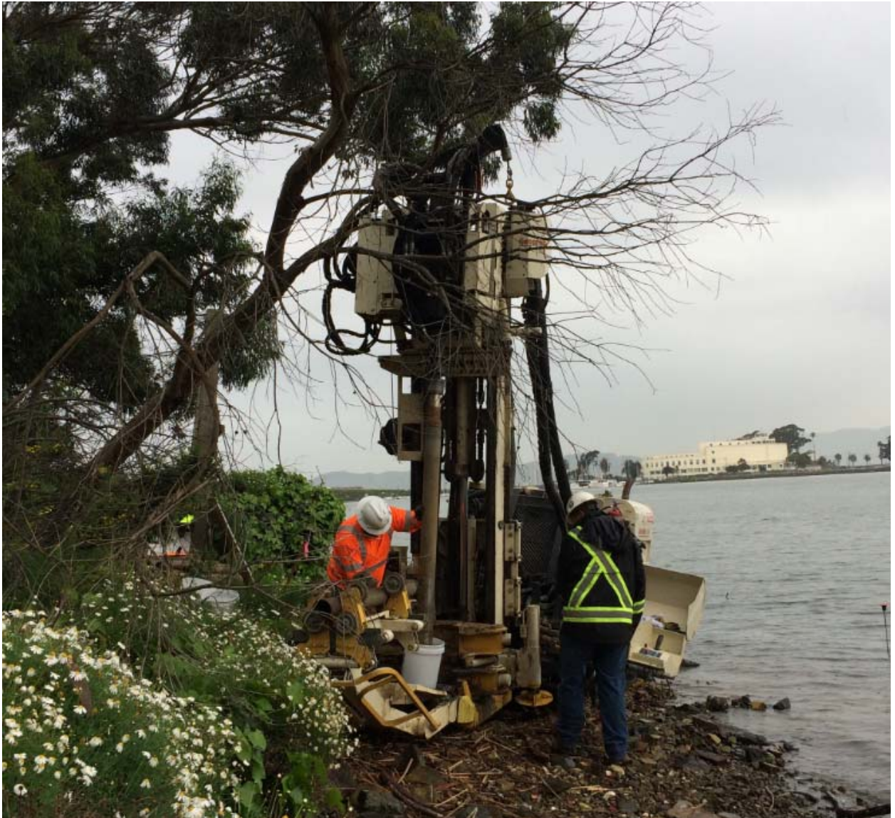
Photograph 2. Collecting the sediment sample for bioassays (0 to 1 feet below surface) at location YF312 using the drill rig.
