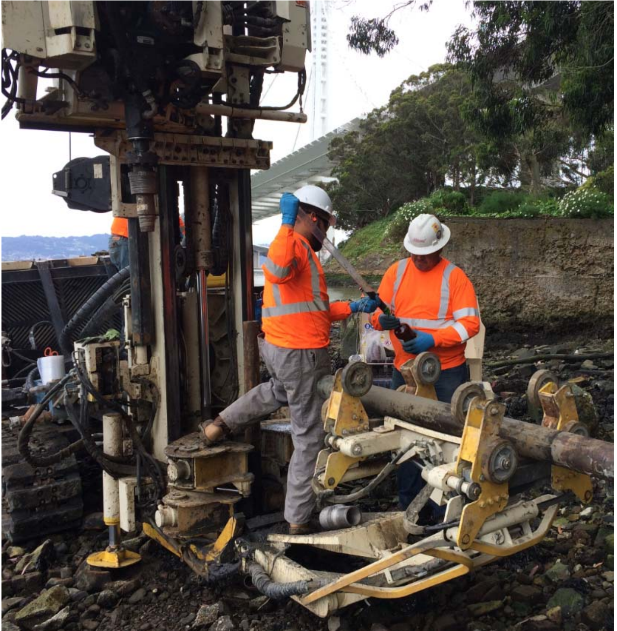
Photograph 4. Collecting the pore water sample at YF308 using a bailer.
