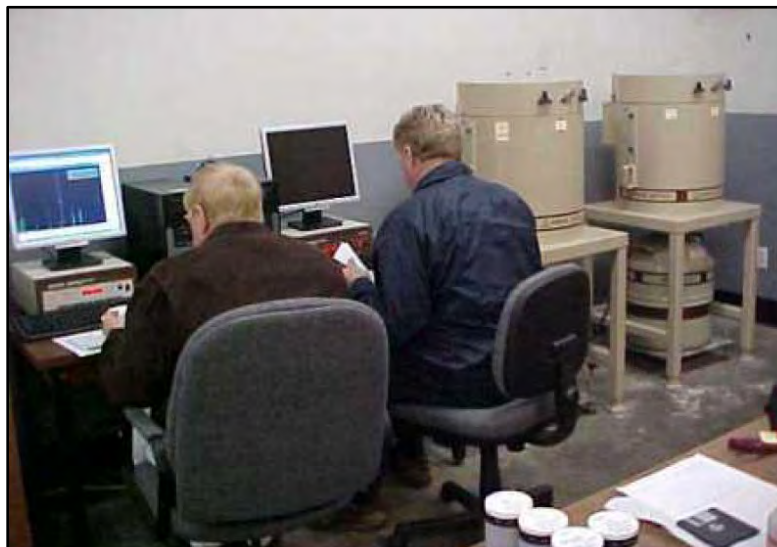
Photo 16 Portable gamma spectrometers in Building 570
