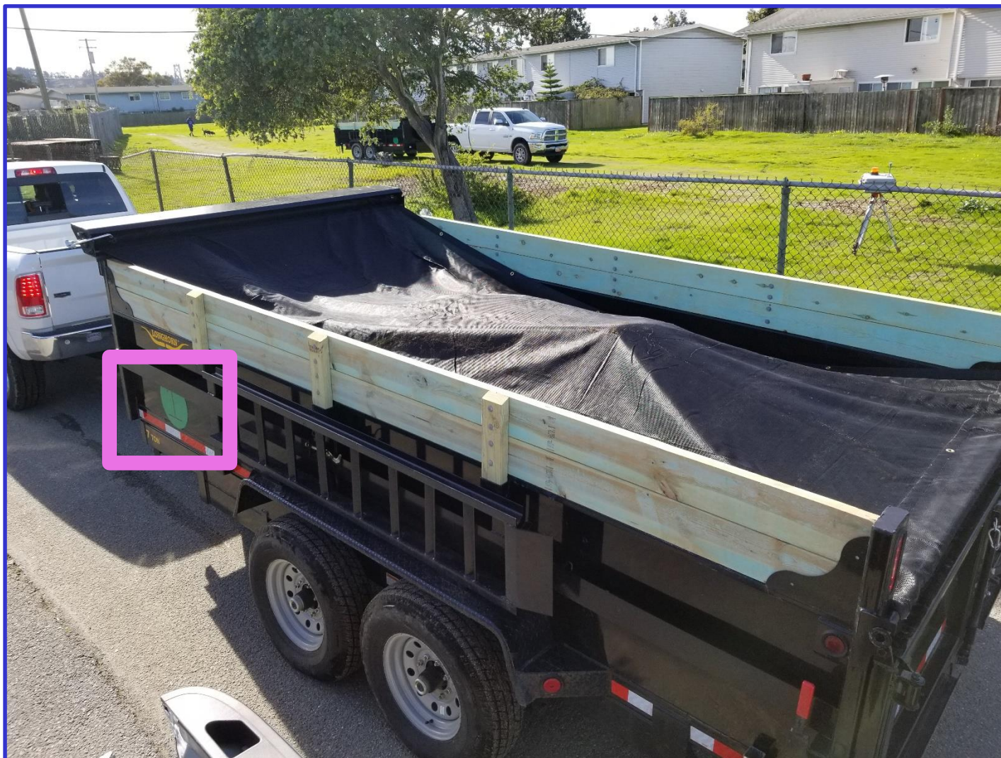
Tarped Trailer Bed Transporting Excavated Soil to Site 32
