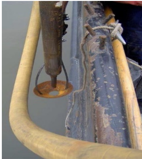
Figure 2-12. Jet Pipe Deployed Over the Side of a Vessel
