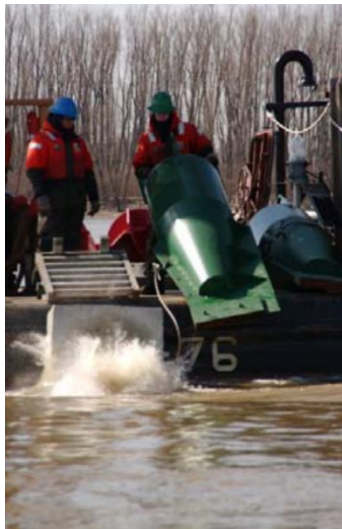
Figure 2-11. Deployment of an ATON from a Dump Board (Aboard a WLR)
