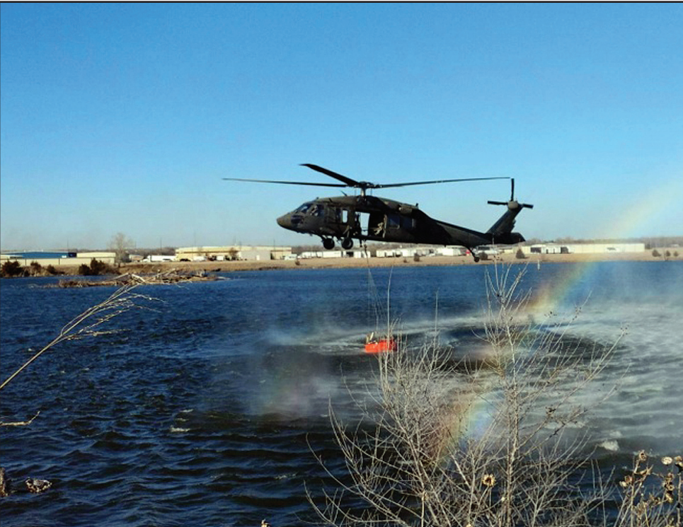
A UH-60 Black Hawk helicopter from the 1st Battalion, 108th Aviation, Kansas National Guard, draws water into the collapsible 660-gallon bucket slung beneath it. The Black Hawk crew was assisting firefighters on the ground battling one of several grassfires in the state in early March. (Photo by Chris Irsik)
