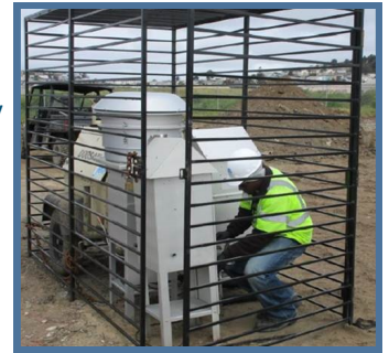
An example of equipment that the Navy uses to collect data on both dust and chemicals in the air
