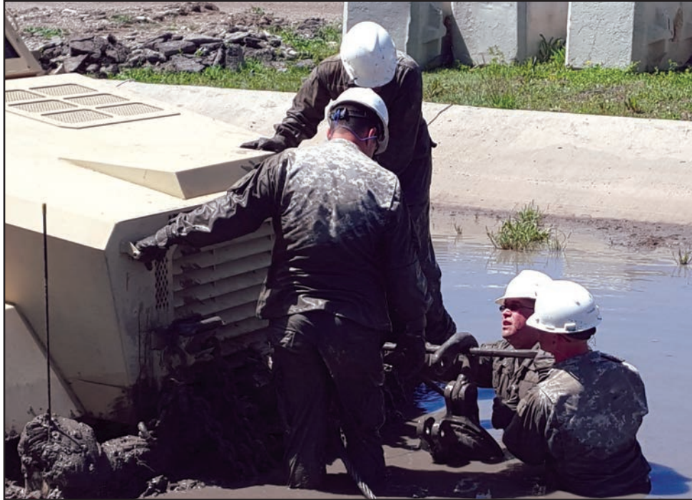
Waist deep in a soupy muck of water and mud, students in the ASIH8 Wheeled Vehicle Recovery Operations Course at the Regional Training Site-Maintenance in Salina assemble the rigging necessary to recover a mired wheeled vehicle. (Photo provided)
