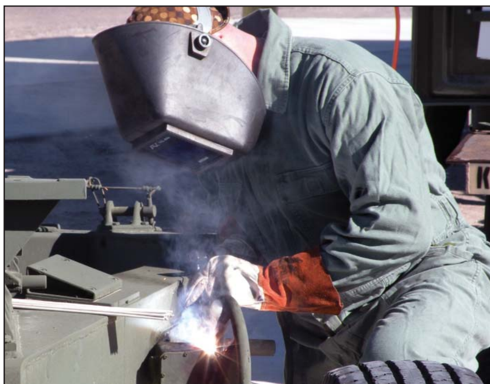
Chief Warrant Officer 2 Kevin Linder, allied trades warrant officer of the 170th Support Maintenance Company, welds a M-102 howitzer to demilitarize it for a military memorial in Scott City, Kan., Nov. 2, 2013. (Photo by Spc. Nancy Baez, 170th Support Maintenance Company)
