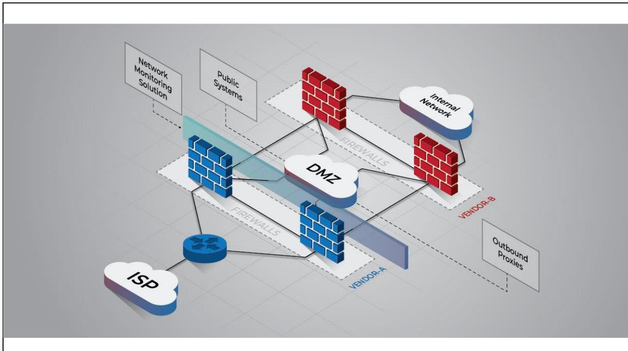
Figure 1: Network perimeter with firewalls and a DMZ
