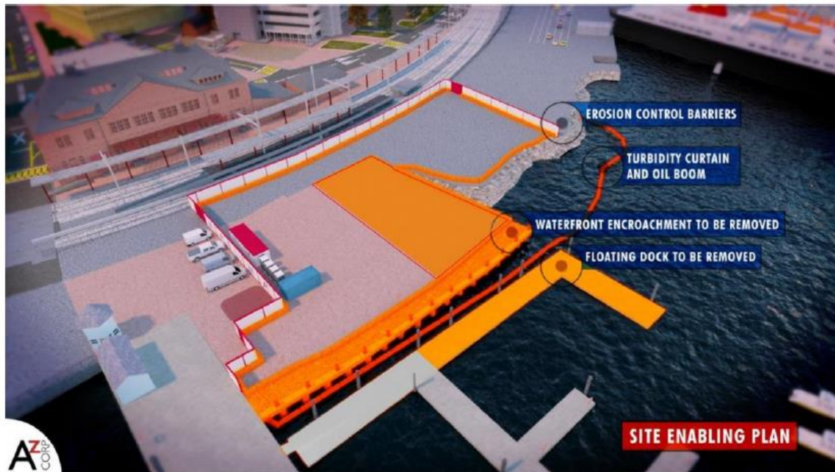
Figure 2.3-13: Waterfront Encroachment Removed
