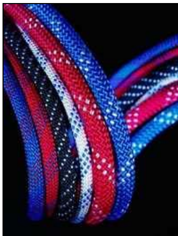
Photo 3-2 – Close-Up View of Kernmantle Rope of Various Sizes
