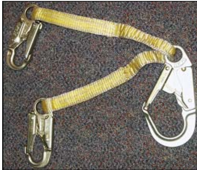
Photo 2-4 – Webbing Work Positioning Lanyard with 3/4" Locking Snaphooks on Each End and a Large 2 1/4" Locking Snaphook for Fastening to Structure
