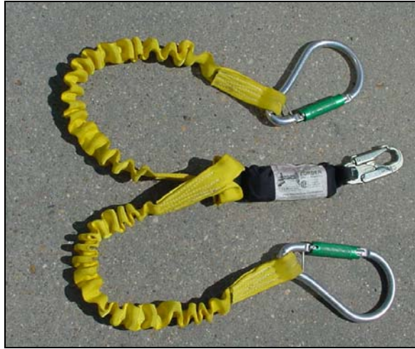
Photo 2-5 – Fall Arrest Lanyard with a Shock Absorber "Pack" and Locking Carabiners for Fastening to the Structure
