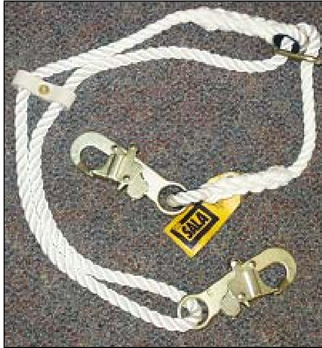
Photo 2-3 – Adjustable Rope Work Positioning Lanyard with 3/4" Locking Snaphooks
