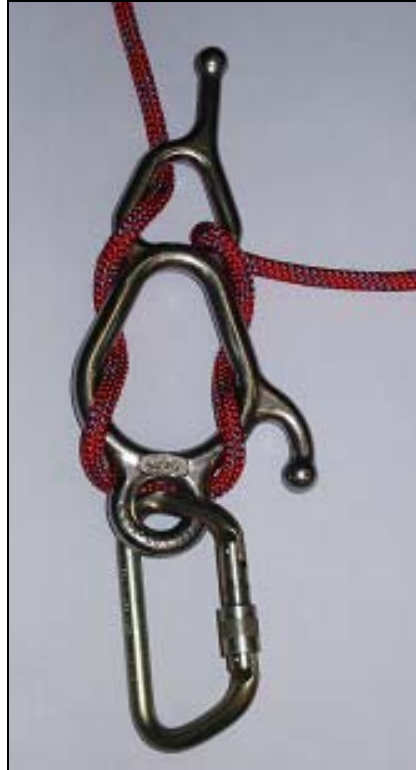
Photos 3-7 and 3-8 – Unrigged (on Left) and Rigged Fisk Descender (on Right)
