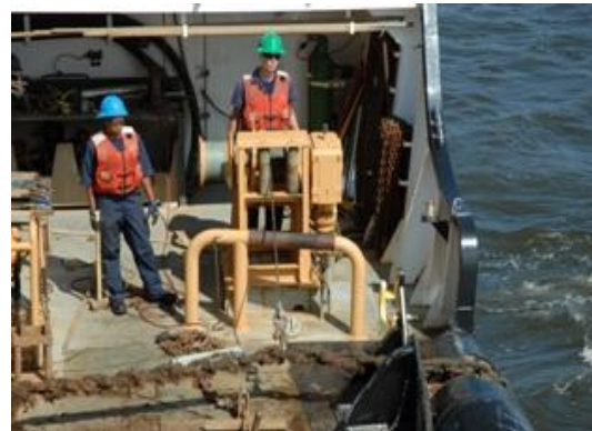
Figure 9-4 Hogging into the Stopper
