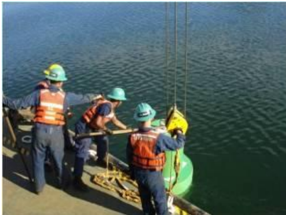
Figure 10-1 Hooking into the Buoy
