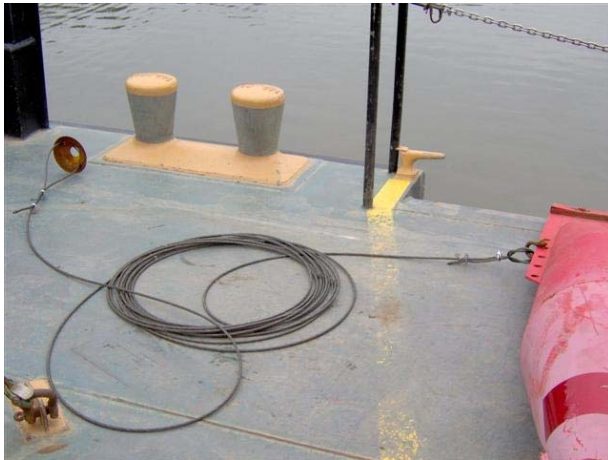
Figure 11-7 Jet Cone Mooring on Deck
