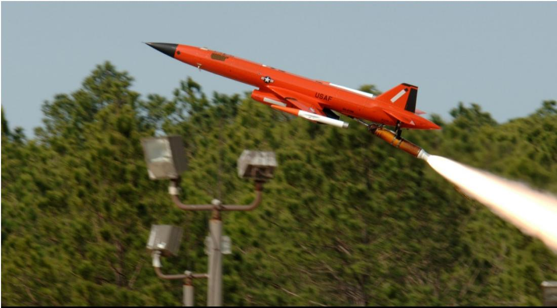
(U) Figure 3. BQM-167A Target Drone
