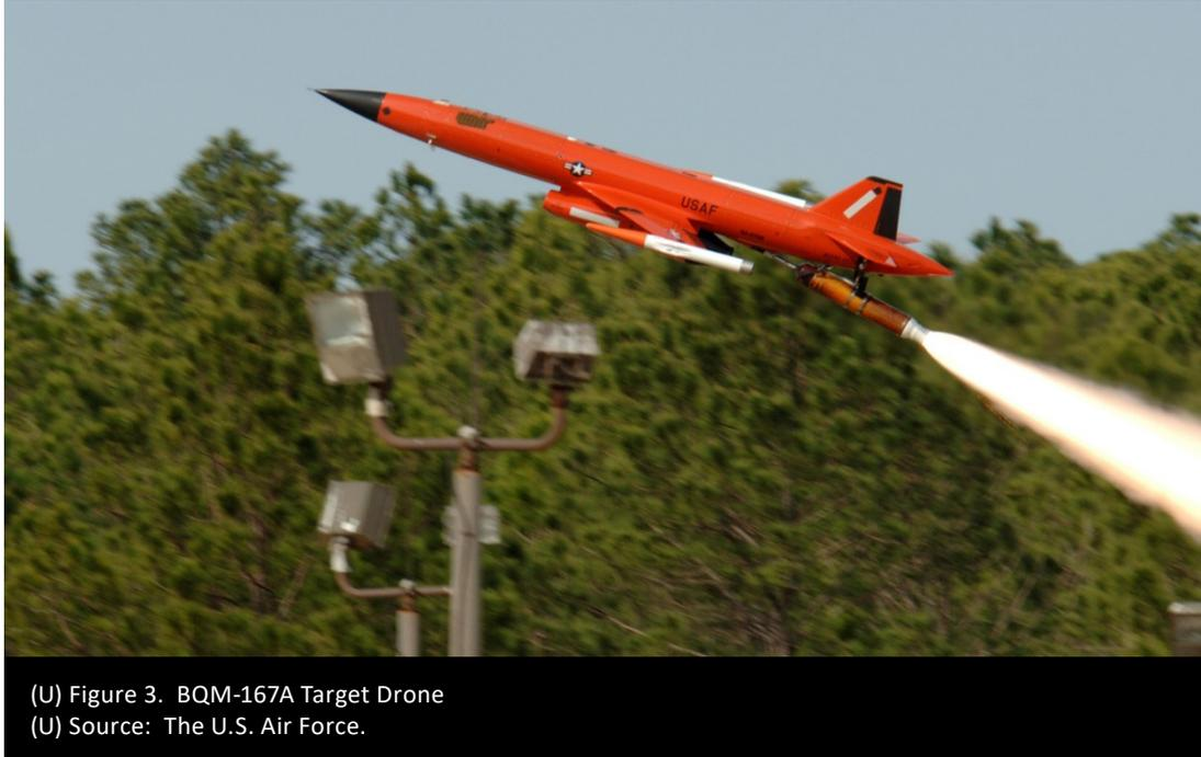
(U) Figure 3. BQM-167A Target Drone
