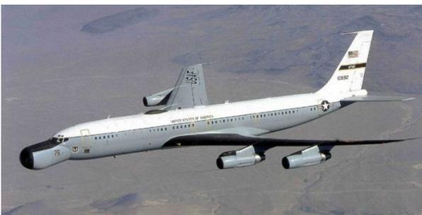
EC-135E, a mobile tracking and telemetry platform to support the Apollo space program and other unmanned space flight operations.
