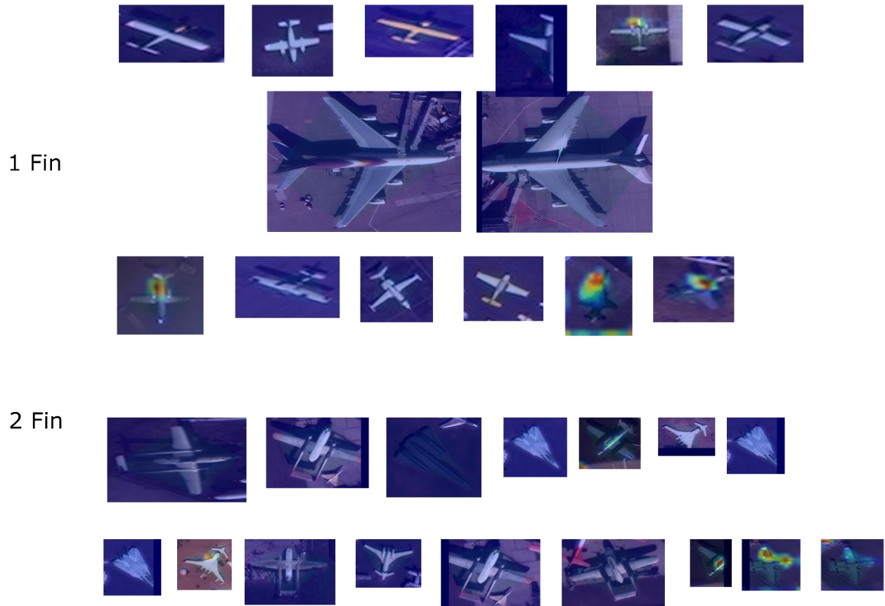
Figure 8 – Example explanations for a surrogate white-box classifier that predicts the number of tail fins. This surrogate model doesn’t seem to be working correctly. Notice that there are few images that have hot-spots where GradCAM shows a high gradient.
