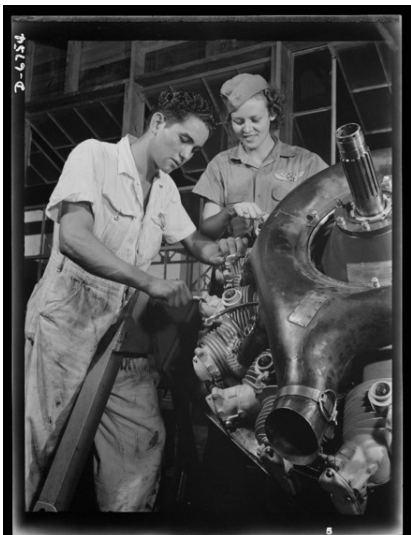
Now an expert mechanic, Mary J. Farley shows a NYA trainee how to repair a Wright Whirlwind motor. (Library of Congress)
