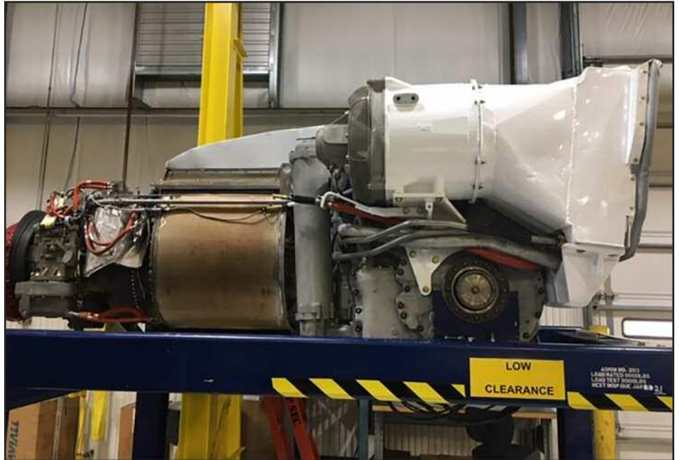
**A completed Full Up Power Pack, consisting of AGT 1500 engine and X1100 3B cross drive transmission, awaits installation into an M1 Abrams tank.**
