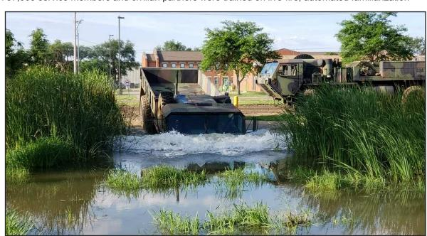
An M977 cargo vehicle is driven into the mire pit at the Regional Training Site - Maintenance as part of the ASI H8 Wheeled Vehicle Recovery Course. Course students will use a M984A2 recovery vehicle, seen in the background, to extract the cargo vehicle from the pit.
