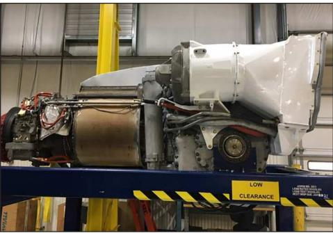
A completed Full Up Power Pack, consisting of AGT 1500 engine and X1100 3B cross drive transmission, awaits installation into an M1 Abrams tank.
