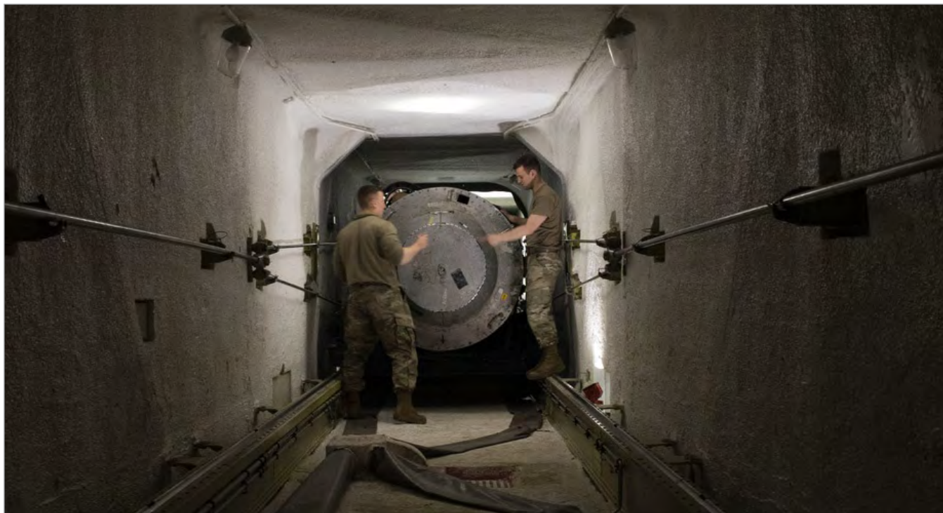
341st Missile Maintenance Squadron personnel securely place a cover on the front of the stage-one booster of the Minuteman III ICBM at the missile handling facility on Malmstrom Air Force Base, Montana, on April 20, 2021.
