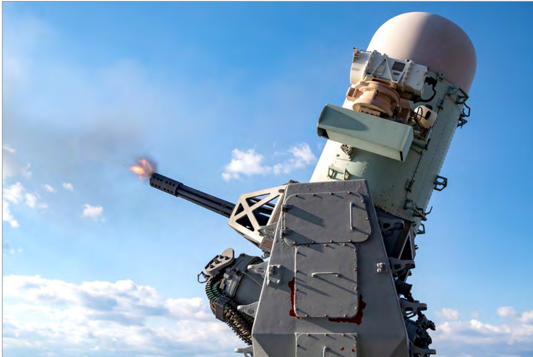
(U) Figure 3. Phalanx Close-in-Weapon System in Operation (U) Source: The U.S. Navy.
