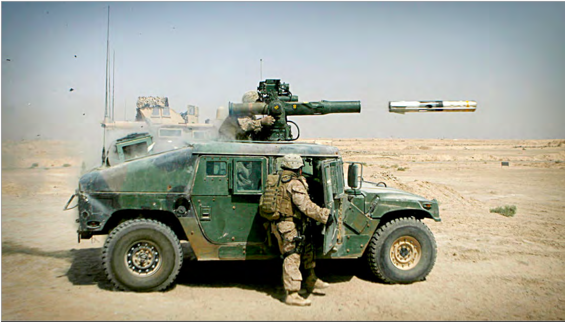
(U) Figure 13. Tube-Launched, Optically Tracked, Wireless Guided Missile Mounted on a Military Vehicle (U) Source: The U.S. Army.
