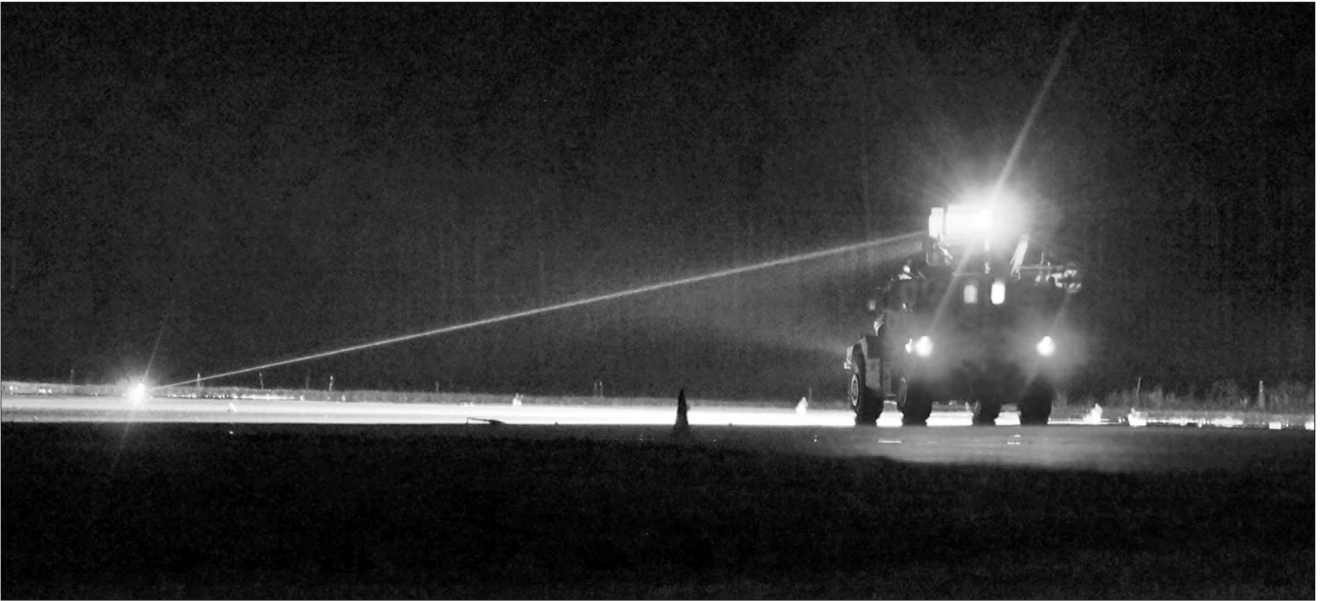
A Recovery of Airbase Denied By Ordnance (RADBO) vehicle, uses a laser to safely detonate and clear unexploded ordnance. The Air Force Life Cycle Management Center's Agile Combat Support Directorate will field 13 RADBOs by April of 2023. (U.S. Air Force photo)
