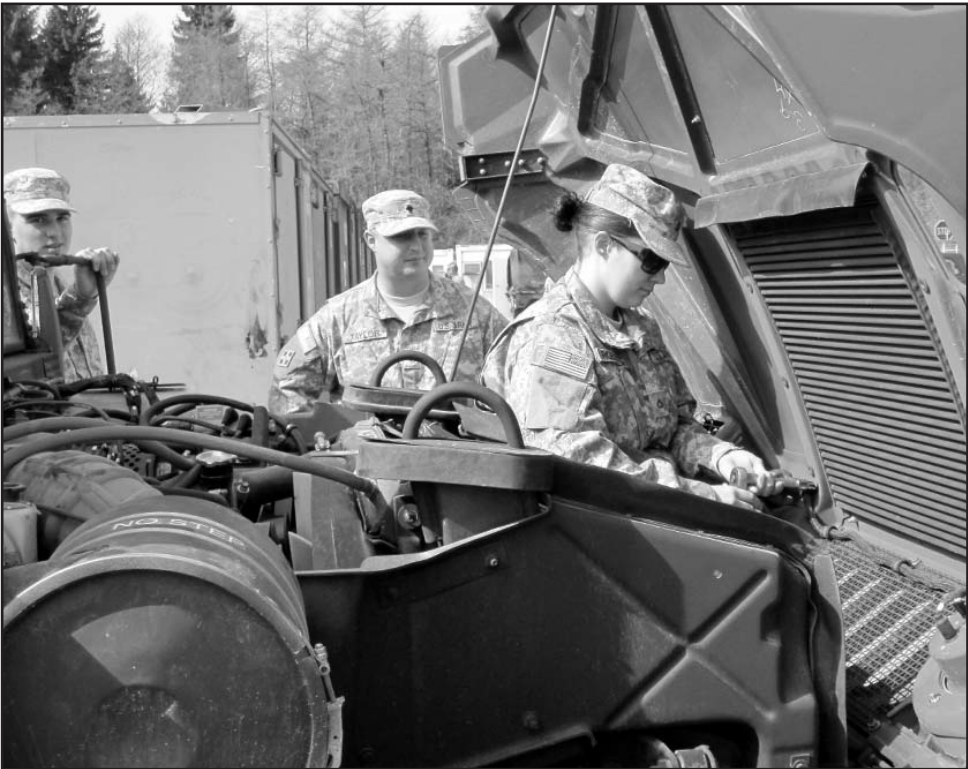
Pvt. Jessie Ryherd (left), Spc. Steven Taylor and Pfc. Tamara Roberts install a new wiring harness on a HMMWV in Hohenfels, Germany. Ryherd, Taylor and Roberts are with the Kansas National Guard's 891st Engineer Battalion. (Photo by Spc. Maureen McWilliams, UPAR, 242nd Engineer Company)
