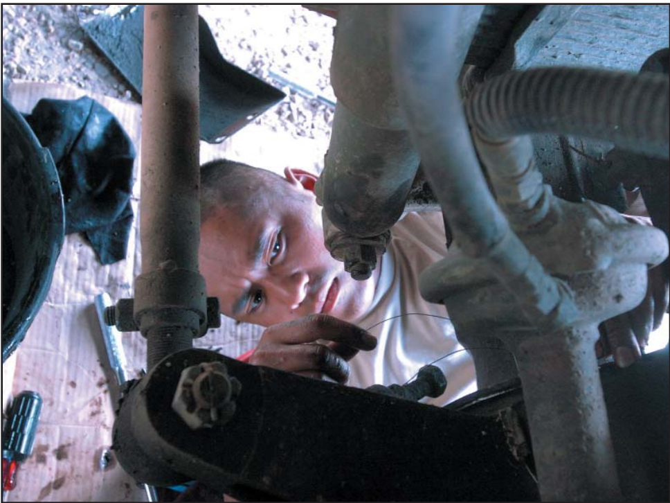
Sgt. Sovoeung Pok, a mechanic with Headquarters and Headquarters Company, 2nd Battalion, 137th Infantry, replaces the grease boot on a five ton truck. Pok deployed to Louisiana in support of relief efforts after Hurricane Gustav ravaged the state, leaving scores without power and water. (Photo by Sgt. 1st Class Phillip Witzke, 105th MPAD)
