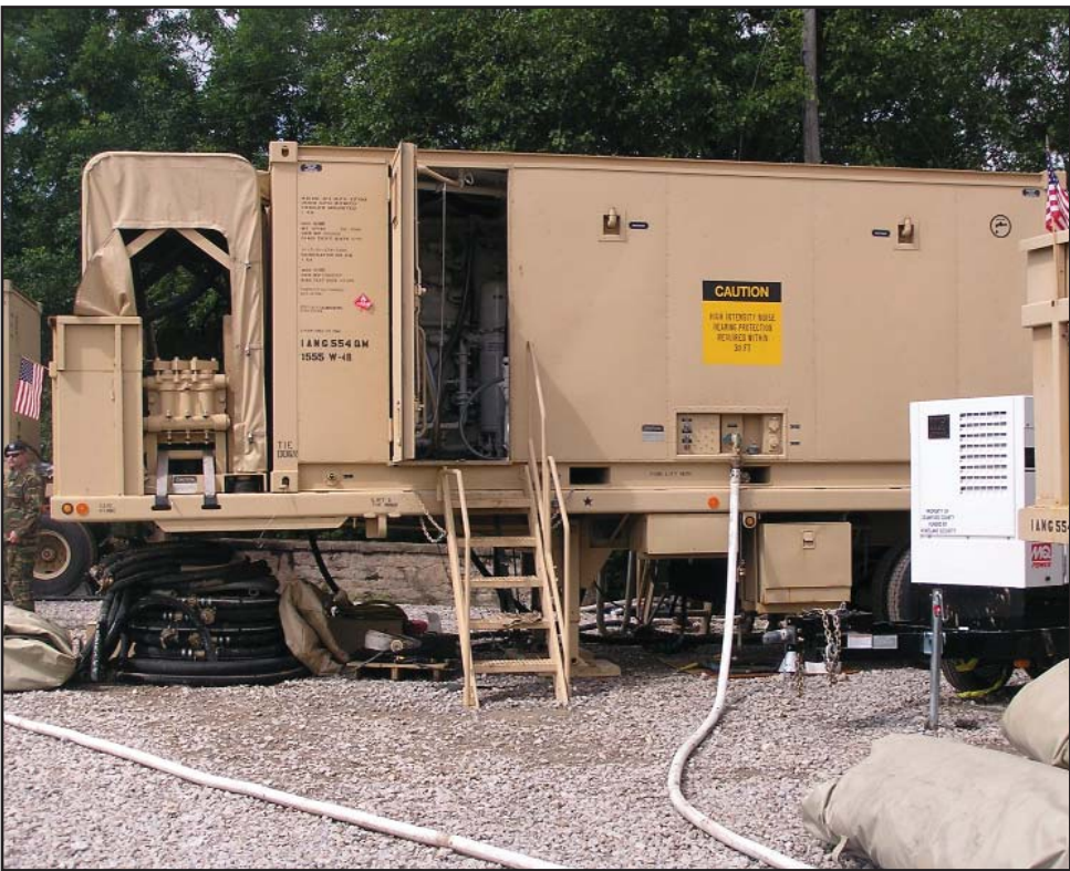
Four Reverse Osmosis Water Purification Units like this supplied fresh drinking water to the people of Fredonia after their water plant was shut down due to flooding. (Photo by 1st Lt. Sean Linn)
