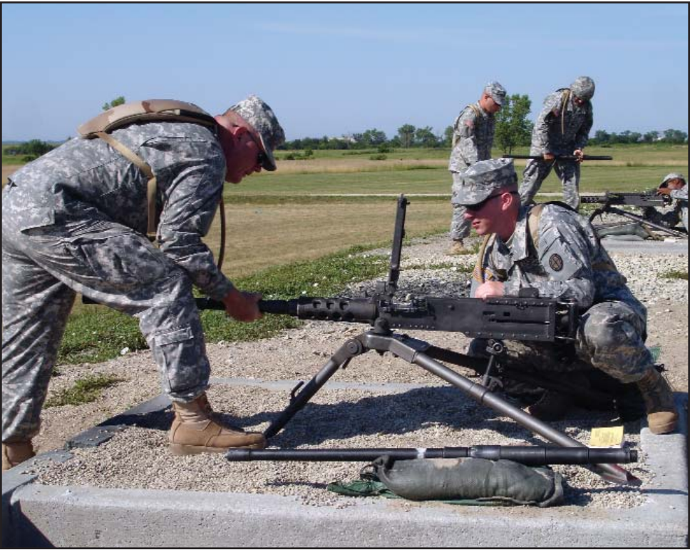
Changing the barrel and adjusting the spacing between it and the receiver is one of the tasks gun crews must complete to qualify on the .50 caliber machine gun. (Photo by Sgt. Michael Mathewson, UPAR)
