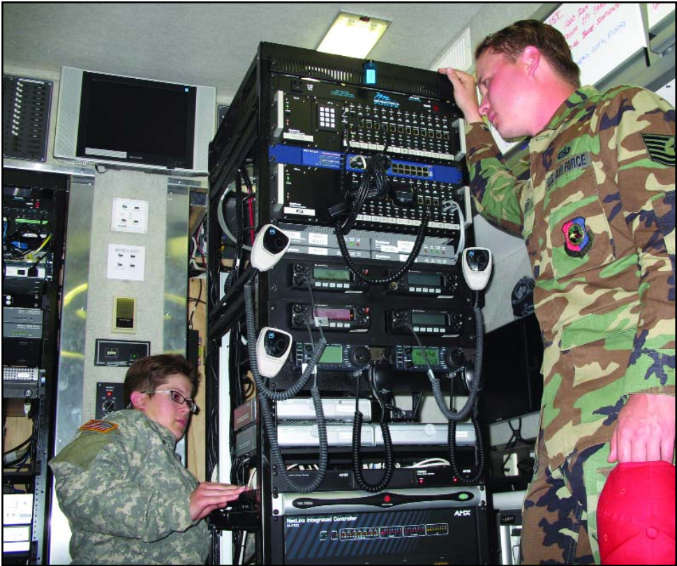
Pfc. Georgia Schafer performs an adjustment on the ACU-1000 as she explains its communication capabilities to Tech. Sgt. Matt McCoy, a photographer with the 184th Air Refueling Wing. (Photo by 1st Sgt. Carl Mar, 105th Mobile Public Affairs Detachment)
