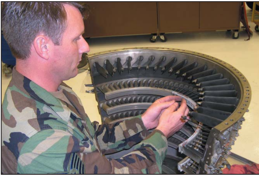
Tech. Sgt. Ray Antal repairs a stator case at the 184th Air Refueling Wing Engine Shop.
