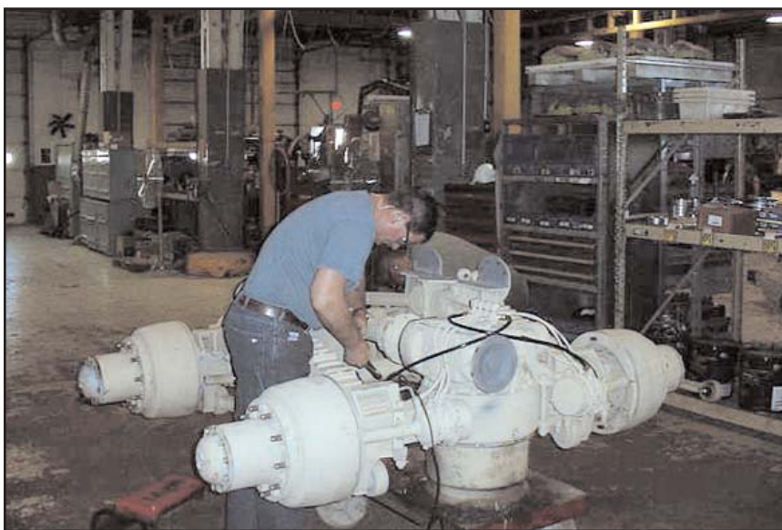
RSMS employee Kenneth McCabe installs ABS (anti-lock brake system) on a rear axle assembly.
