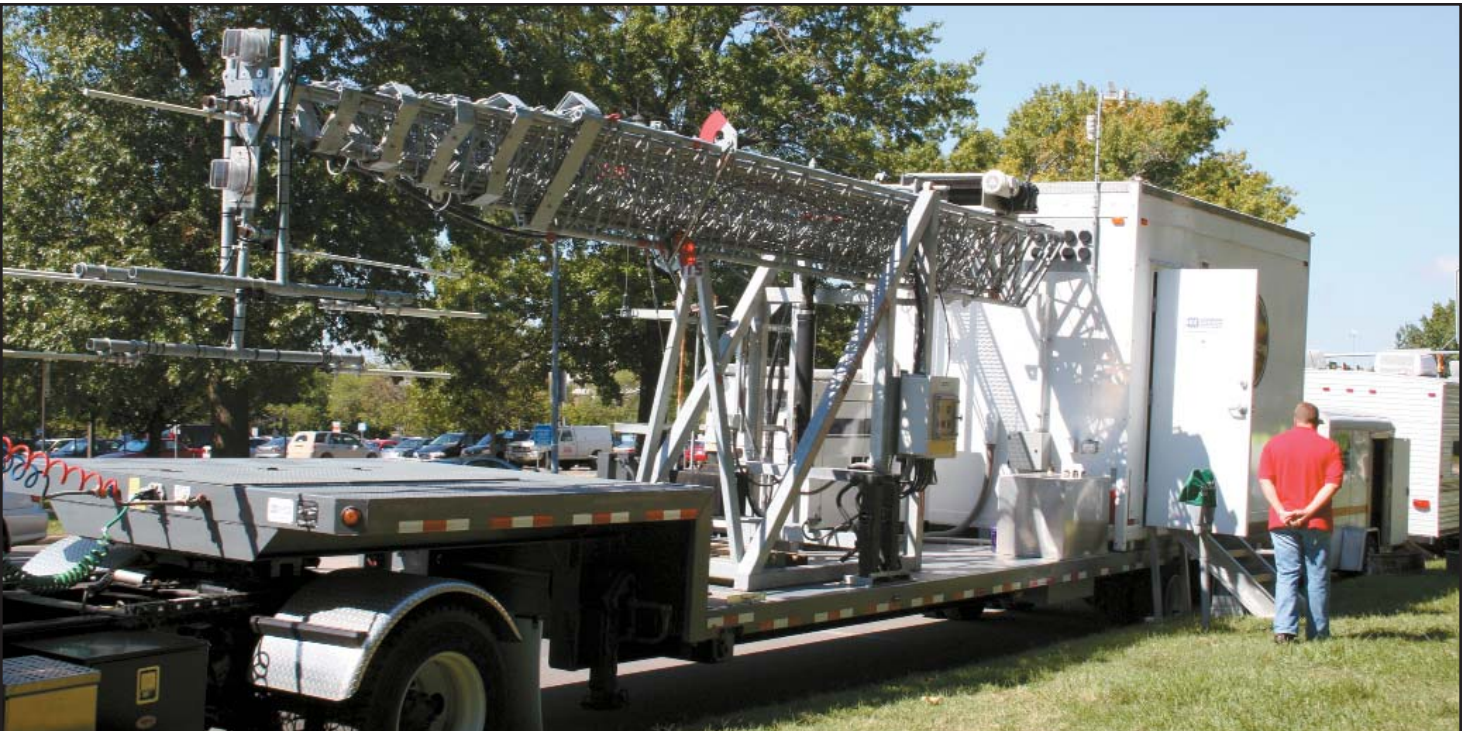
The Communication On Wheels vehicle is a mobile communications center that can be used in emergency situations to keep lines of communications open between first responders and civil authorities during a large-scale disaster.
