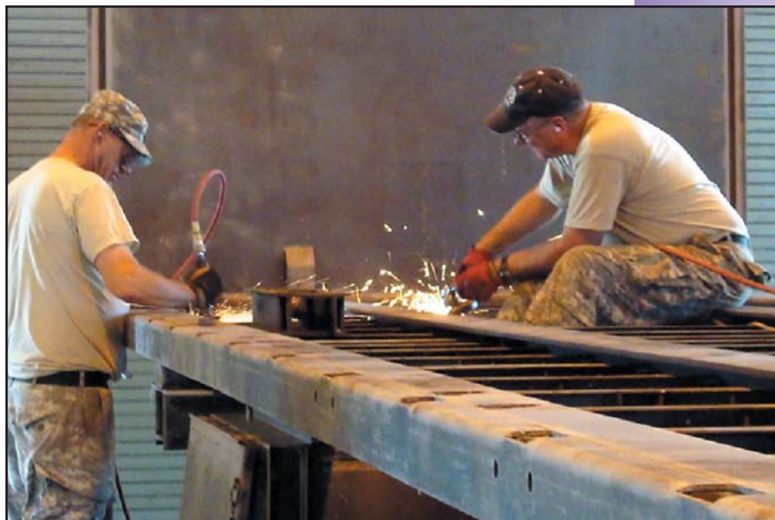
Sgt. 1st Class Jerrold Lyne and Staff Sgt. Joseph Sterling complete fabrication repair during the rebuild of a M872A2 Trailer assigned to the 731st Transportation Company.
