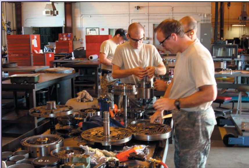
Spc. Robert Wunderle and Staff Sgt. John Peterson start the rebuild process on a M654 transmission. The MATES rebuilt over 150 similar transmissions during Fiscal Year 2008.
