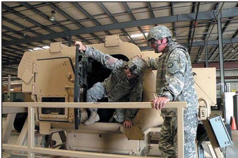
Soldiers of the 35th Infantry Division practice proper egress techniques from a humvee in a roll-over simulator.
