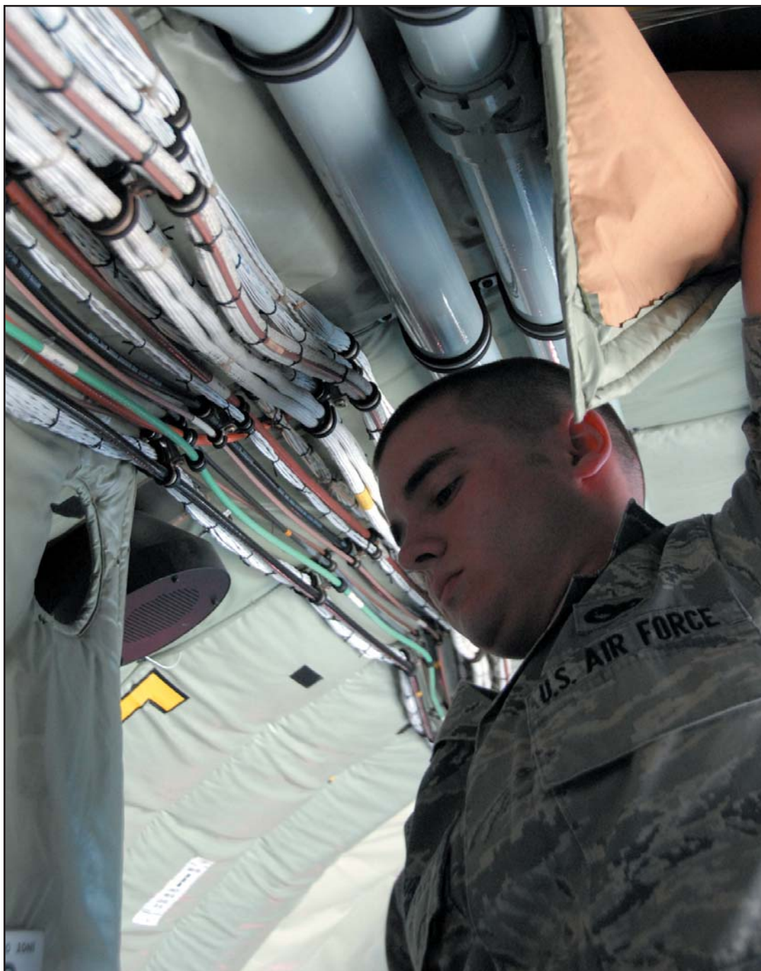
Senior Airman Jesse Reid adds power outlets to a KC-135R. The added outlets allow the tanker to airlift three times as many medical patients requiring electrically powered equipment.
