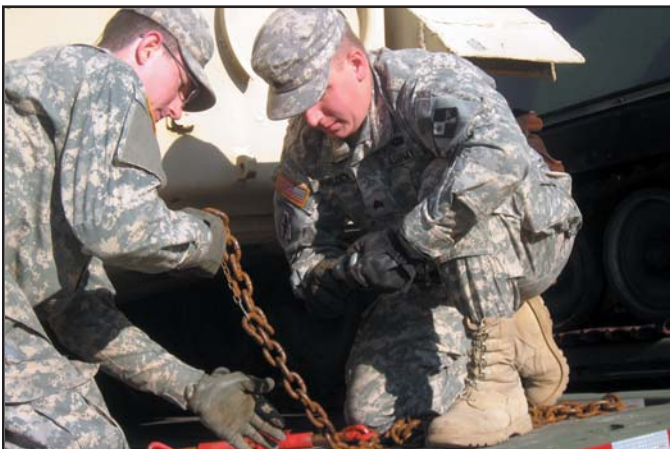
Sgt. Peter Parlock (right) teaches Spc. Jessie Worthington how to properly chain and binder an M113 hull at Camp McCrady, S.C., during the 731st Transportation Company's annual training.
