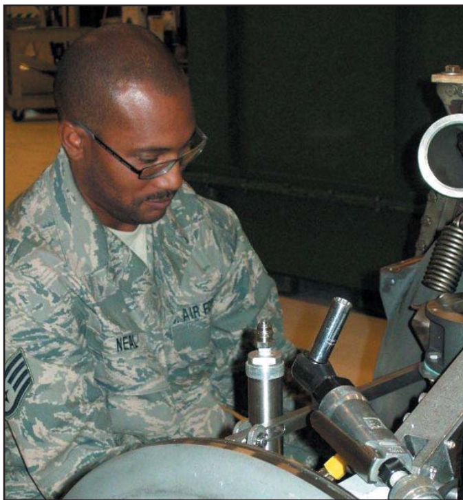
Staff Sgt. Mario Neal works on an AGT 1500 turbine engine at the Advance Turbine Engine Army Maintenance site.
