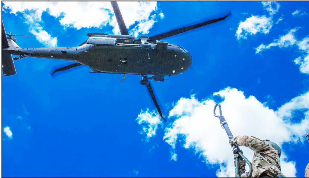
Soldiers of the 1st Battalion, 108th Aviation practice connecting a slingload to a UH-60 Black Hawk helicopter.
