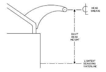
Figure P-2: Representation of davit head height for calculating lowering speed
