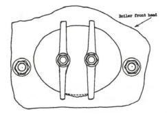
Repair consists of thorough cleaning or grinding to sound metal, magnetic particle testing to ensure no fractures exist and building up of original thickeness by welding.
