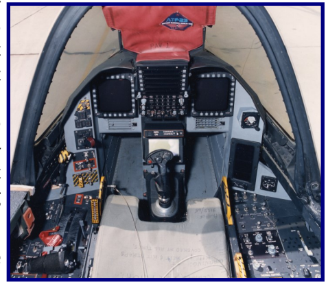
The cockpit of the YF-23 is based around the F-15E Strike Eagle. Two 5" x 5" Multi-Purpose Color Displays (MPCD) occupy a large portion of the main instrument panel.
