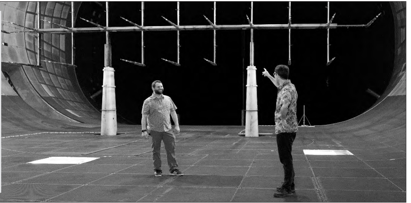
Kyle Lukacovic, left, a test engineer at the National Full-Scale Aerodynamics Complex, and Paul Gilles, an NFAC instrumentation engineer, look around the 40-foot by 80-foot Wind Tunnel of NFAC at Moffett Field, California, where a flow characterization study was recently completed. During the multi-phased effort, updates were made to the existing flow calibration and characterization in the tunnel. Pictured behind Gilles and Lukacovic is the test rig used for the flow evaluation. NFAC is an operating location of the 716th Test Squadron, 804th Test Group, Arnold Engineering Development Complex. (U.S. Air Force photo) (This image was altered by obscuring a badge for security purposes.)
