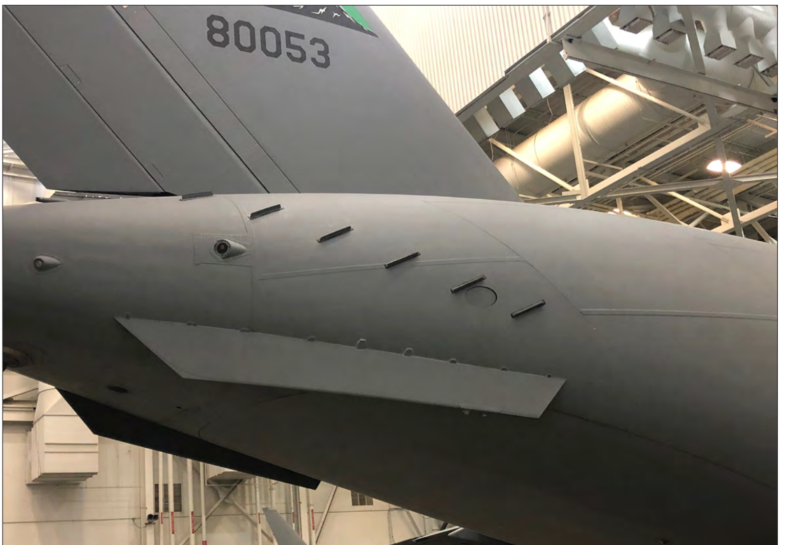
The drag reduction devices known as microvanes are shown on the aft-end of a C-17 Globemaster III at Joint Base Lewis-McChord, Washington. (U.S. Air Force photo)
