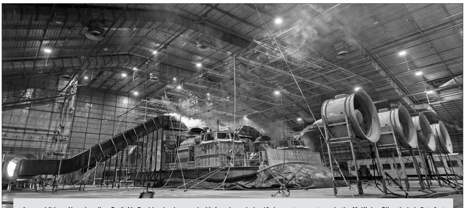
An amphibious Navy Landing Craft Air Cushion is showered with freezing rain in -10-degree temperatures in the McKinley Climatic Lab Oct. 6 at Eglin Air Force Base, Florida. MCL, an operating location of the AEDC 717th Test Squadron, is used to conduct climatic testing of various military and commercial systems. The LCAC, from Naval Surface Warfare Center Panama City, underwent climate testing in the Lab's large chamber. (U.S. Air Force photo by Samuel King Jr.)
