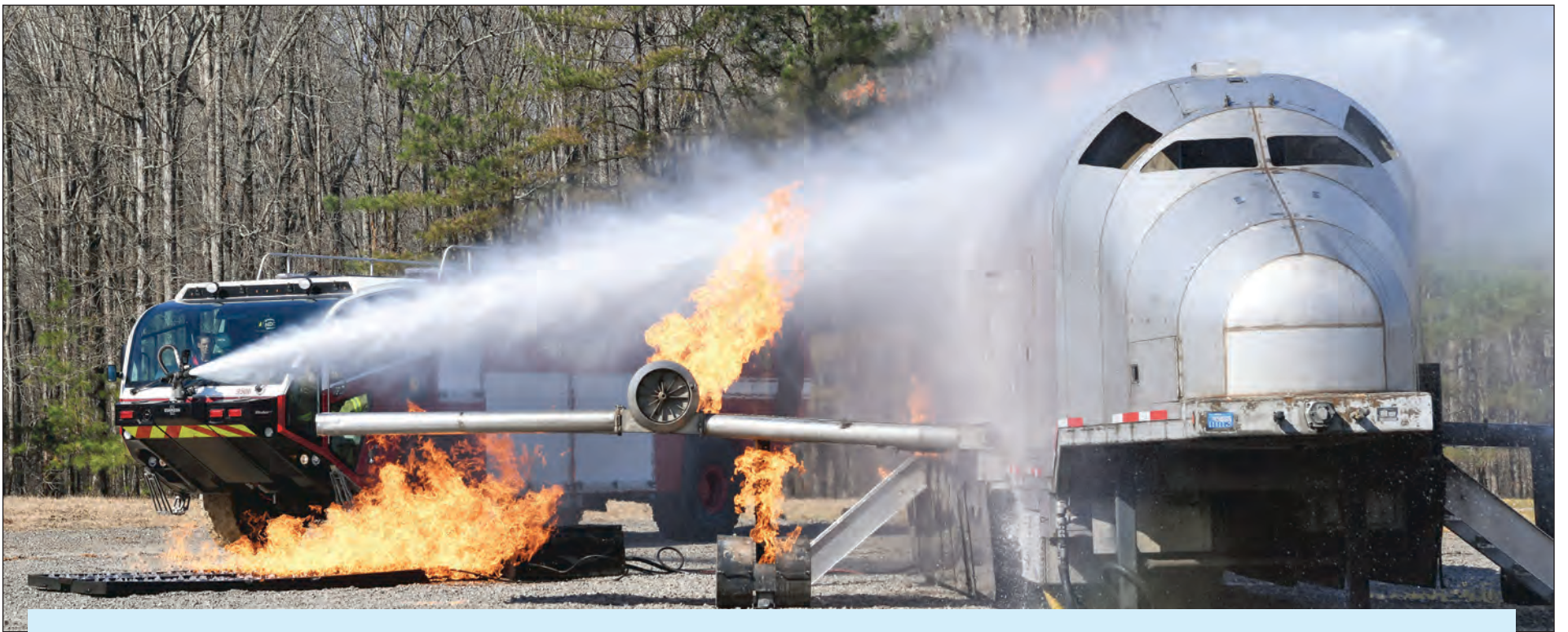
Arnold Air Force Base Fire and Emergency Services personnel operate a bumper turret spraying water as they train March 3 on aircraft rescue and firefighting techniques at the base. (U.S. Air Force photo by Jill Pickett)
