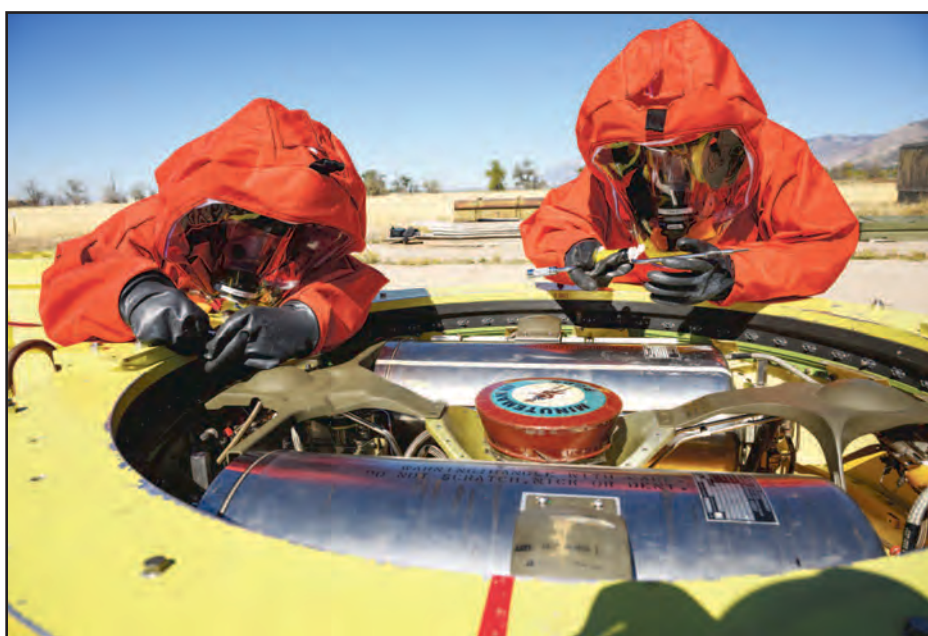
Members of the Missile Mishap Response Team work on a Minuteman III inert guidance system during a training event at Hill Air Force Base, Utah, Oct. 4. The highly-specialized team responds to any number of situations involving an ICBM (except the warhead) where technical procedures do not exist, or the loss of life is possible. (U.S. Air Force photo by R. Nial Bradshaw)
