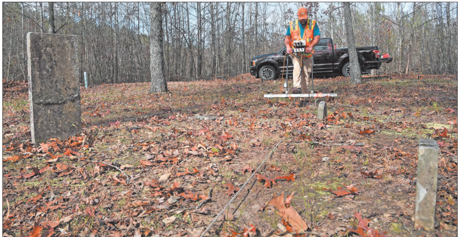
Steve Martin, an archaeologist who specializes in geophysics, uses an electrical resistance meter to survey the Chapel Hill Cemetery at Arnold Air Force Base Nov. 10. The survey can help the archaeologists assess what has happened below the surface in an area. This information can then be interpreted to identify possible graves that were never marked or the markers are no longer in place. (U.S. Air Force photo by Jill Pickett)
