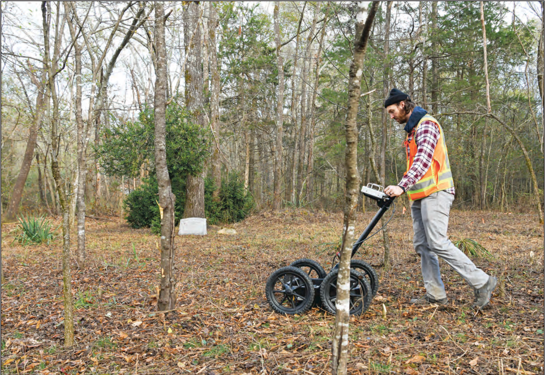
Jacob Jepsen, an archaeologist who specializes in geophysics, operates a ground penetrating radar machine in Rutherford-Shipley Cemetery at Arnold Air Force Base Nov. 10. The GPR data gives archaeologists information about what has occurred below the surface to help detect possible grave locations. (U.S. Air Force photo by Jill Pickett)
