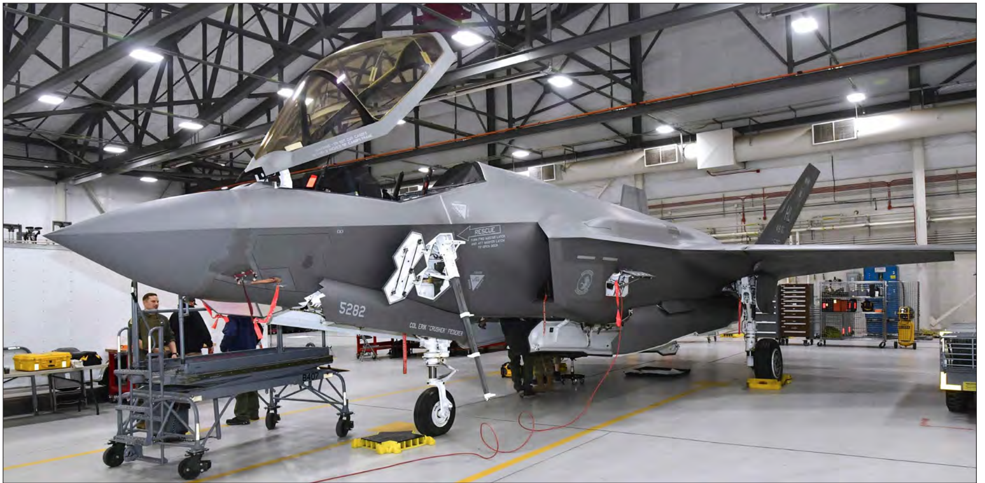
An F-35 Lightning II is equipped with Quick Reaction Instrumentation Package components March 23 Hill Air Force Base, Utah. The QRIP records all data and uploads into a knowledge management system, allowing for faster software development, better reprogramming, and expedited products out to the pilots. (U.S. Air Force photo by Todd Cromar)
