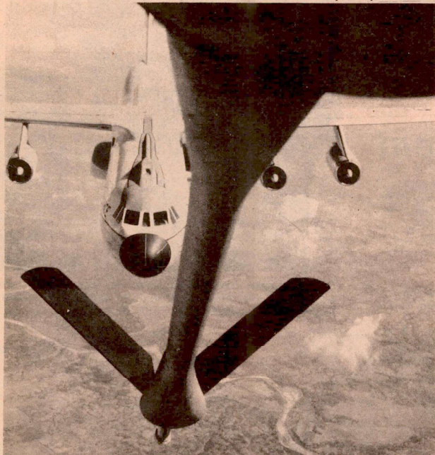
A C-141B Starlifter pulls into its airborne gas station for a flight-extending fill up. Modifications now allow it to be refueled in midair. (U.S. Air Force photograph)
