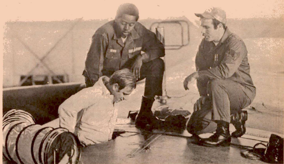
SSgt. William F. Mays, fuels systems technician, 317th Field Maintenance Squadron slips into a C-130 fuel tank access hatch to check on a fuel leak. Assisting him is Amn Gilbert Brown, a fuels systems apprentice with the 513th FMS and SrA Stephen A. Dodson, 317th OMS, the plane's crew chief.
